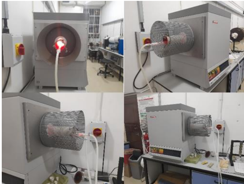
Figure 4.3: CVD Experimental set-up using Carbolite CTF Tube Furnace (Serial No. 21-103513).
