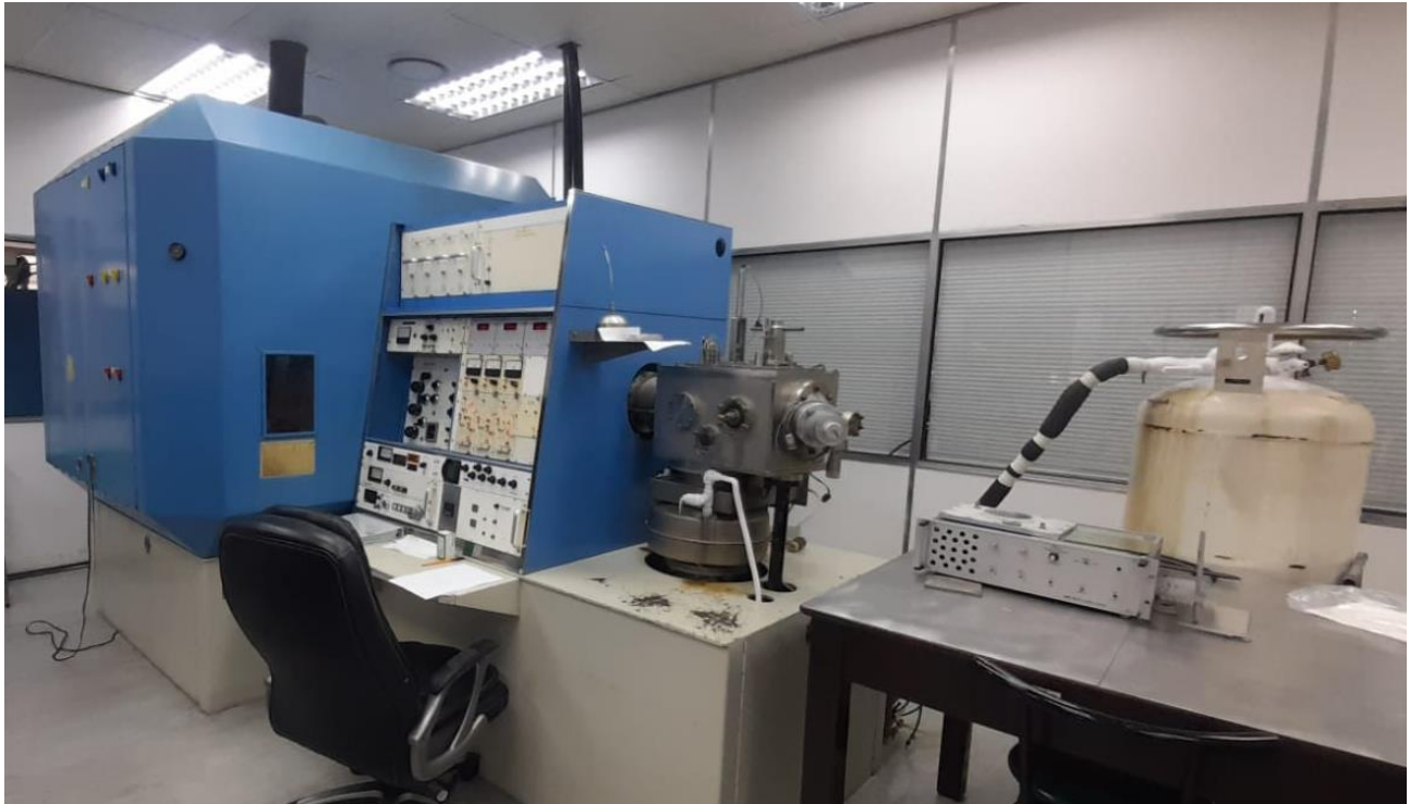
Figure 4.5: Varian-Extrion 200-20A2F ion implanter.
