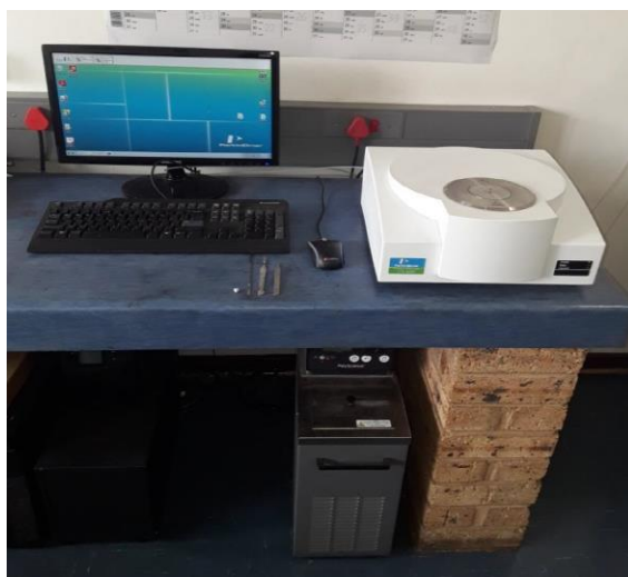
Figure 3.3: Thermal analyzer used for the TGA.
