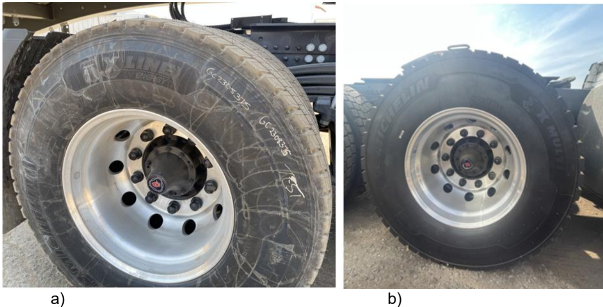
Figure 3.5: Tyres on vehicles used in the study. a) Fleet 650 fitted with Michelin X Line Energy tyres (low-rolling-resistance, green tyres) and b) Fleet 651 fitted with Michelin X Multi tyres (conventional, black tyres).
