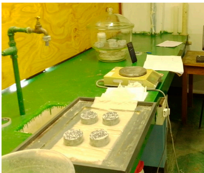
Figure 5. Water sorptivity testing of concrete samples.
