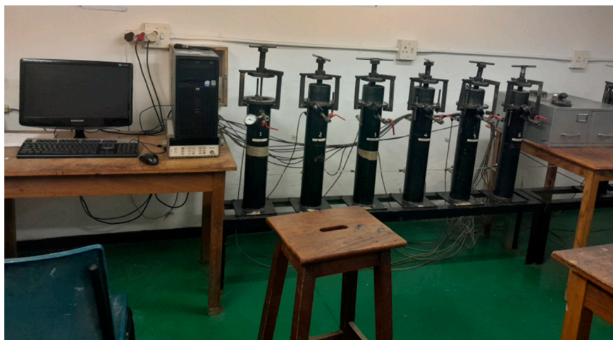
Figure 4. Oxygen permeability cell setup.
