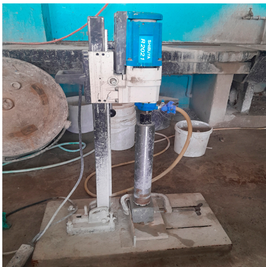
Figure 3. Preparation of sample concrete disc for durability tests.
