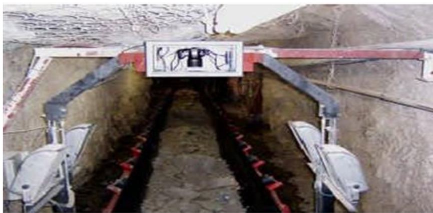
Figure 3.3 Nikon digital camera and lighting system installed over a conveyor at level 74 Kopanang mine (Source: Brink et al., 2008)
