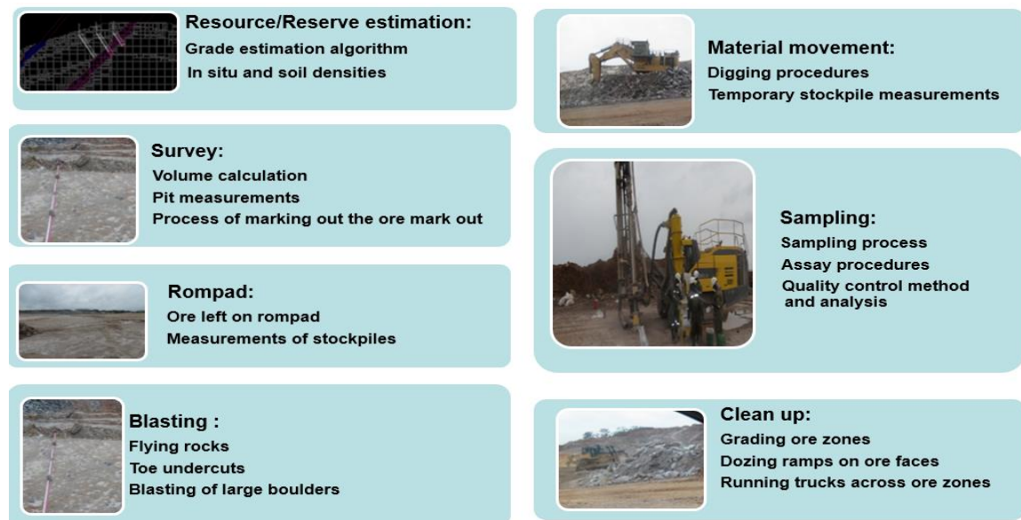
Figure 2.1. Variable components of the MCF for surface mines (Source: Tetteh and Cawood, 2014)
