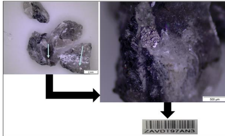
Figure 5.11 Microdots visibility on coarse sample A2 (Source: Researcher, 2016)
