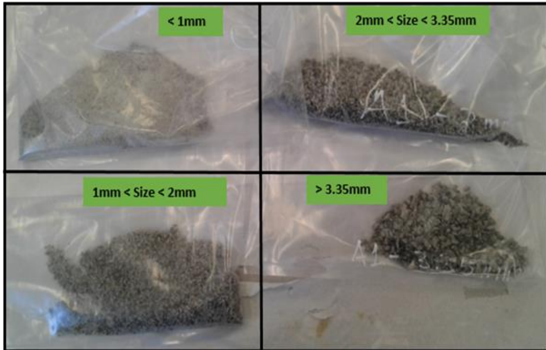
Figure 5.10 Screened samples into various fine sizes (Source: Researcher, 2016)
