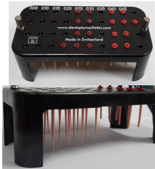
Fig. 3.4 GP cones seated in an endo stand, prior to batch allocation, demonstrating free contact of the entire circumference of the cone for solvent exposure.
