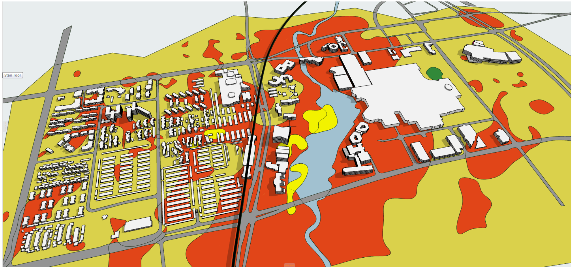
Figure 58_ Existing Built Form on Hazard Areas
