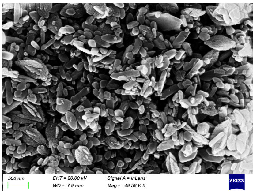
Fig. 3. SEM image of as-synthesized CuO nanoparticles prepared using Novel method at room temperature and without calcination of the synthesized CuO nanoparticles.
