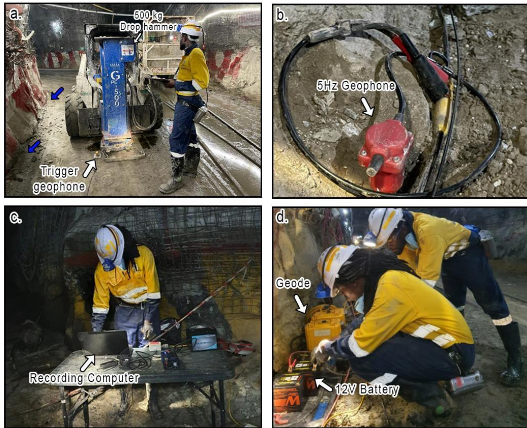
Figure 5.2: A summary of the South Deep Tunnel-1 (SDT1) acquisition setup. (a) The type of source used for the survey with the blue lines showing where the cabled system was, (b) the type of sensor/geophone used, (c) the recording unit setup, and (d) the geode system and the power supply.
