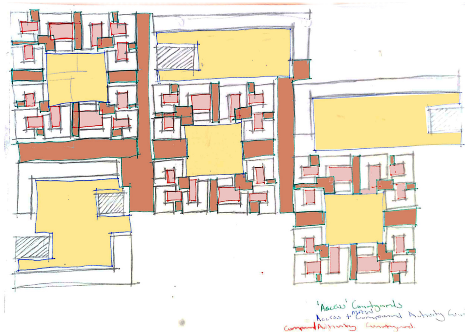
Figure 4.55: The pattern created in Figure 4.54 allows for the development of unique pockets of space with different thresholds of privacy. The brown spaces can be defined as access courtyards. The pink spaces can be access and activity courtyards. These activities being limited to smaller groups that have direct access to the compound. The yellow spaces are access and main activity courtyards where activities for the whole compound (which is a combination of smaller compounds) can occur.
