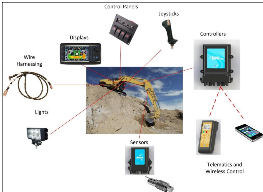
Figure 4.10 How a shovel can be connected to IoT (Gomori, 2016)
