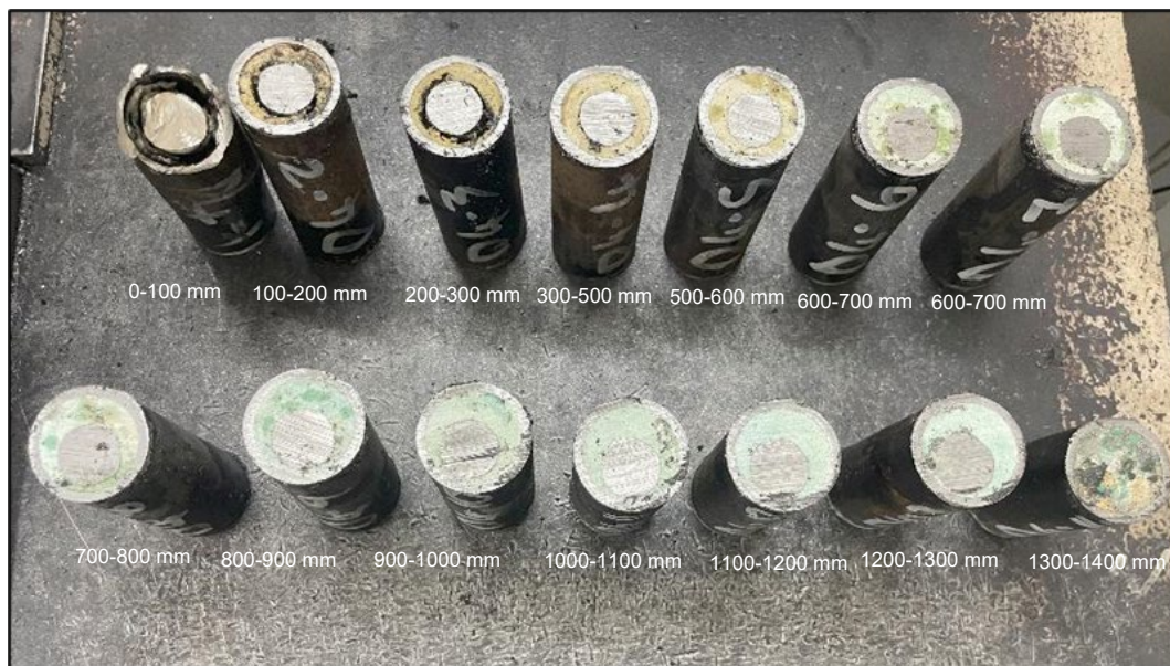
Figure 4-9: Photo showing the extent of impact damage and poorly mixed resin of Sample D4.
