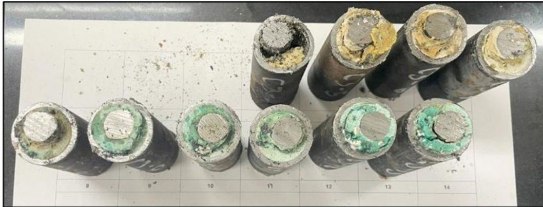
Figure 4-8: Photo showing an example of the condition of Test C samples post-testing.
