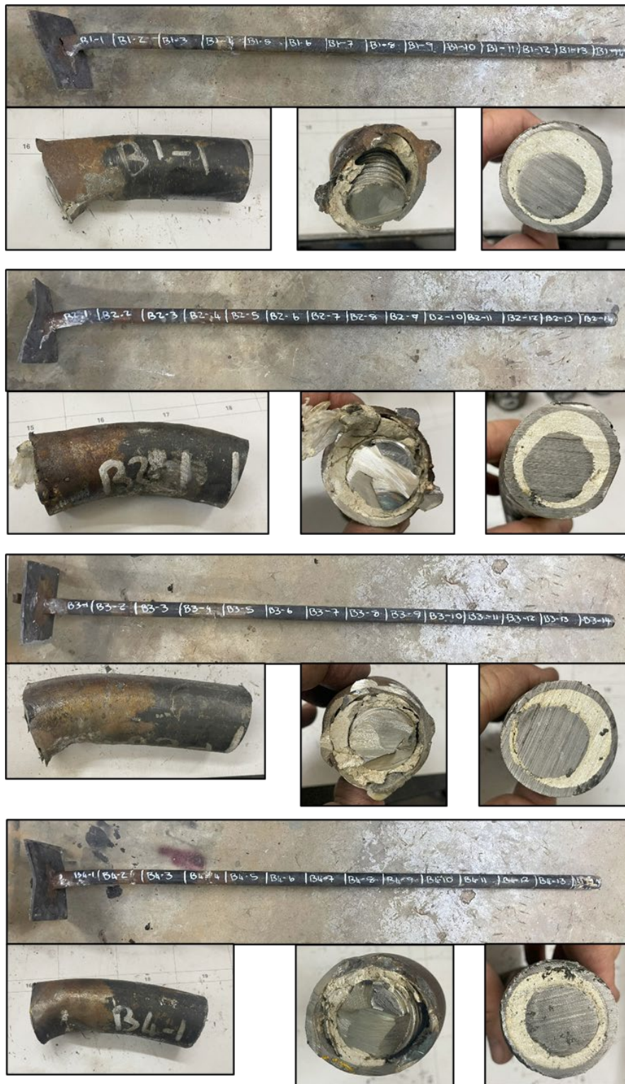
Figure 4-5: Photo showing the damage to the first segment of each test.
