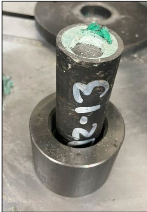
Figure 4-10: Soft, unmixed resin pushed out of the sample, Test D.
