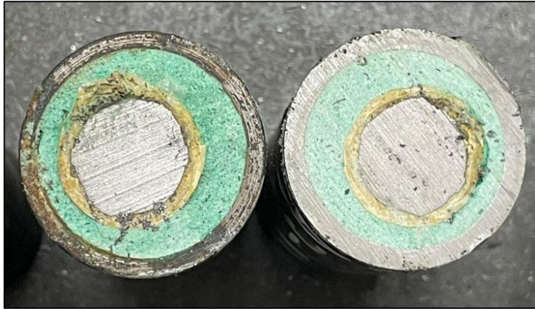
Figure 4-2: An example of gloving observed in samples from Mine A.
