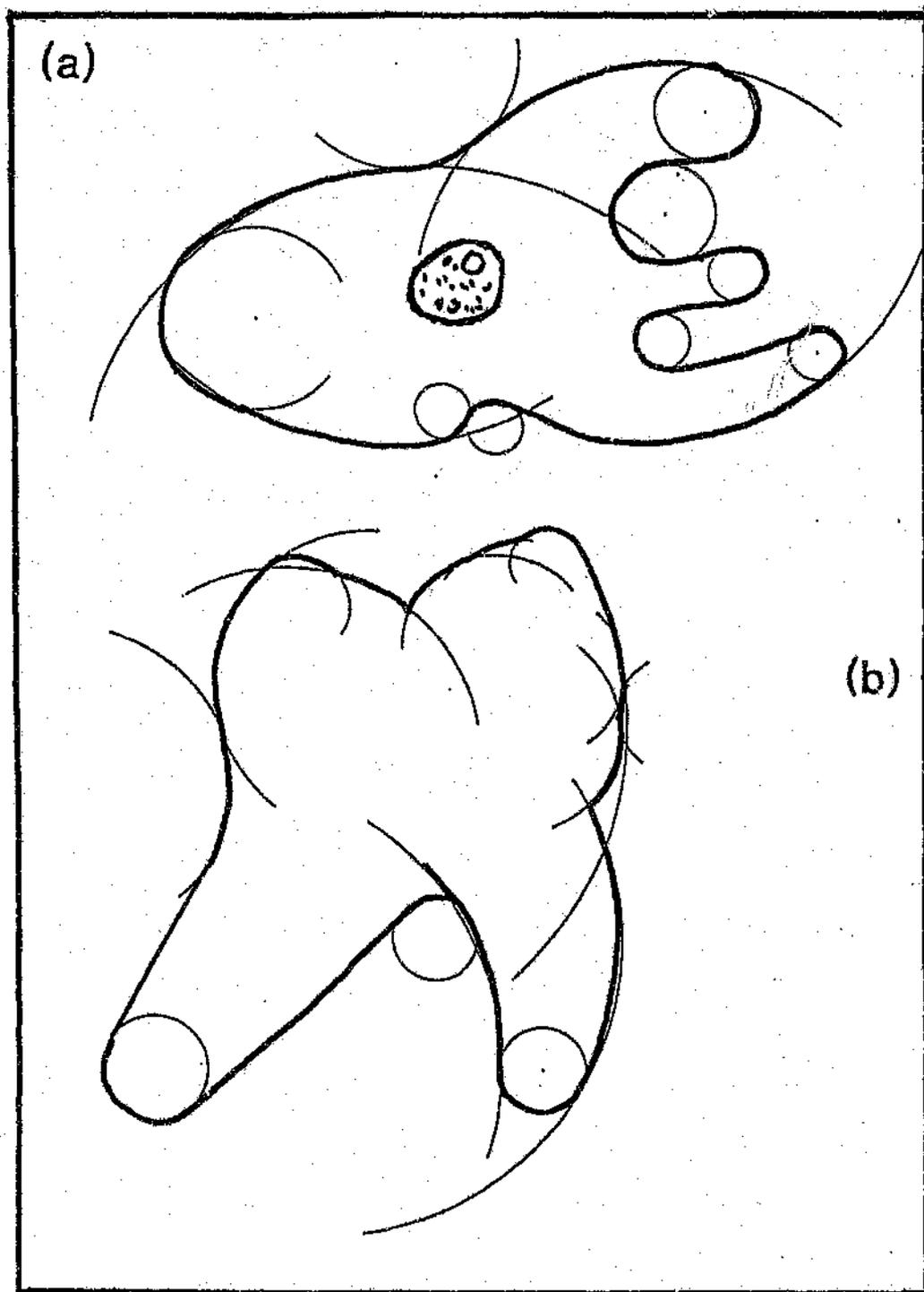
FIGURE 15 - Simplifying compound curves with simple arcs.
