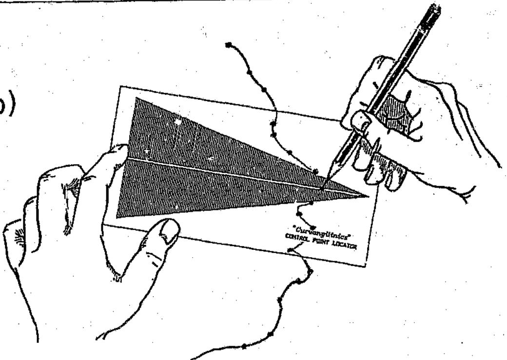
FIGURE 19 - The Control Point Locator (CPL).
