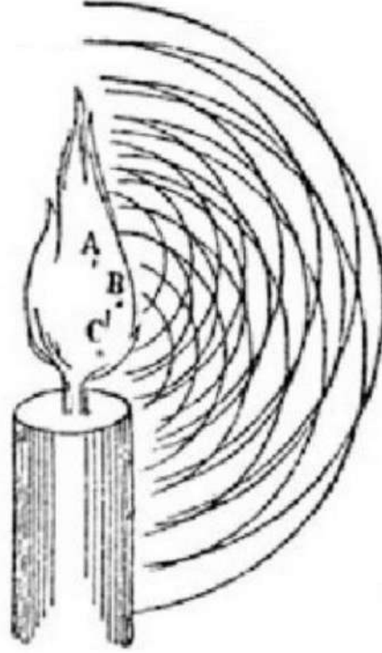
Figure 3.3: An illustration of Huygens' principle - the superposition of elementary waves (after Russer and Russer, 2015 ).
