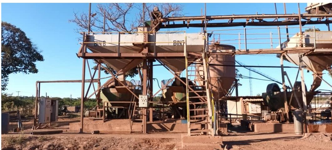
Figure B8 Picture of the 15t surge bins with fine ore
