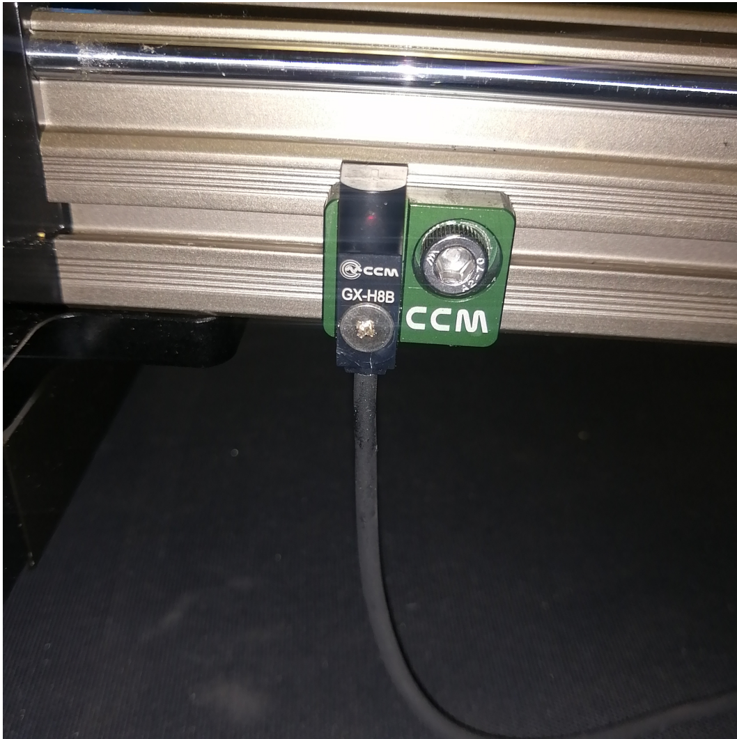
Figure 3.7: The GX-H8B proximity sensor located on the left of the upper linear actuator.
