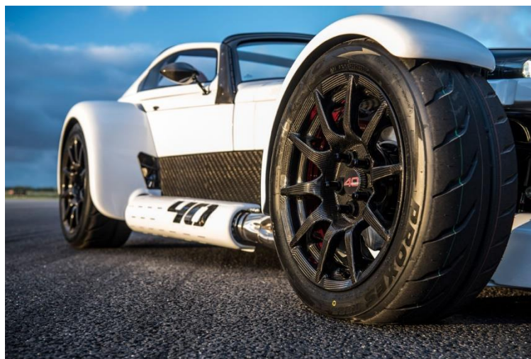
Figure 6-1 Donkervoort D8 GTO-40 with CFRP wheels developed in this study [19]
