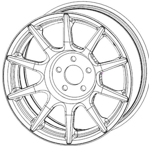
Figure 2-2 CAD geometry of the tested wheel
