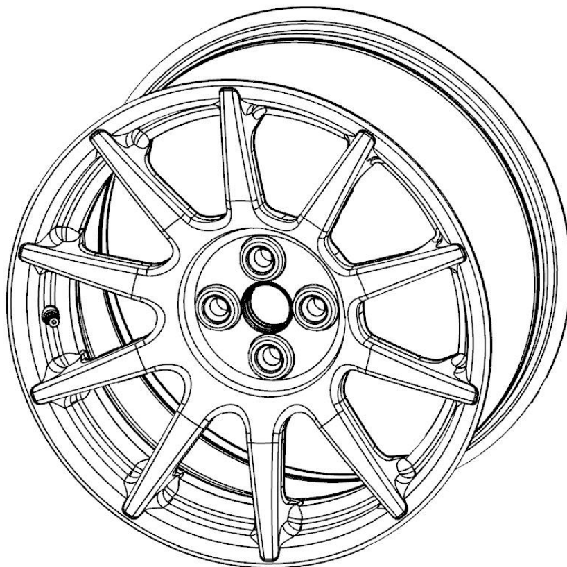
Figure 5-1 CAD model of the wheel used for thermal testing
