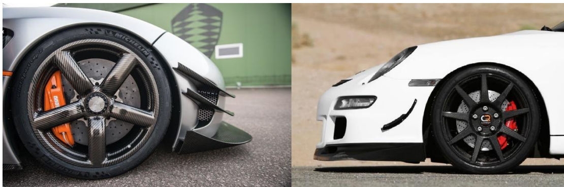
Figure 1-1 (a) Koenigsegg CFRP wheel (L) (b) Carbon Revolution CFRP wheel (R)
