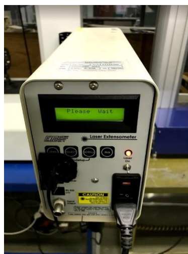
Figure 3-8 Laser extensometer used for material testing
