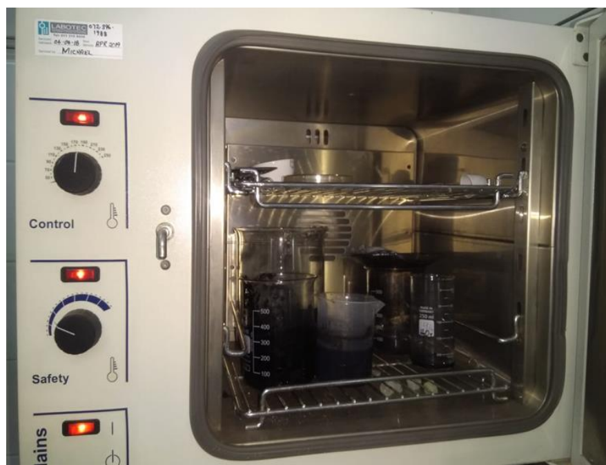
Fig 3.7: Carbon chemical activation in an electric oven
