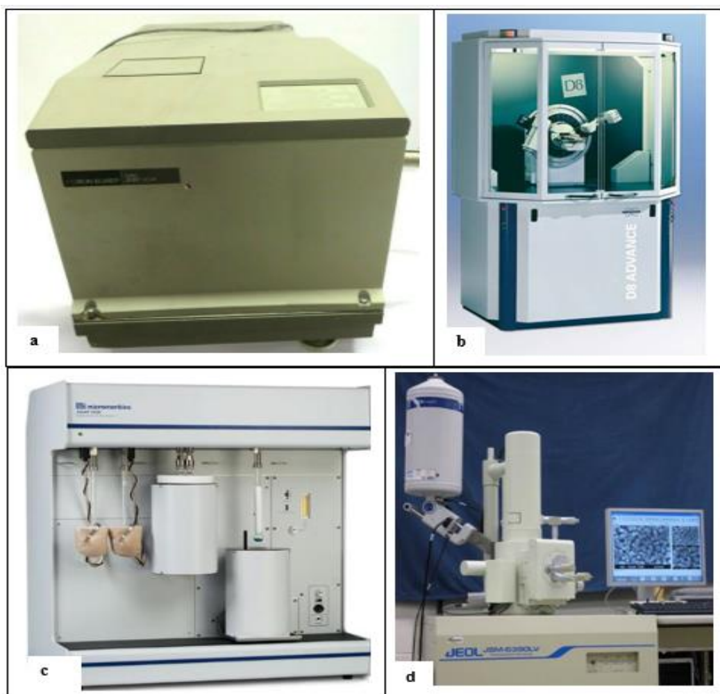
Fig 3.3: Analytical equipment used for (a) FTIR (b) XRD (c) BET (d) SEM/EDX
