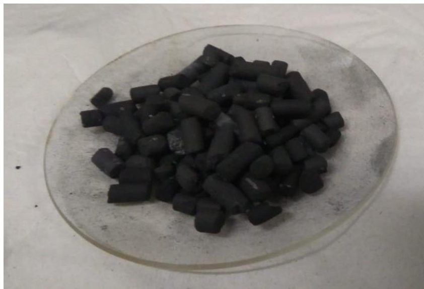
Fig 3.2: Picture of saturated commercial grade activated carbon sample from Reclite.
