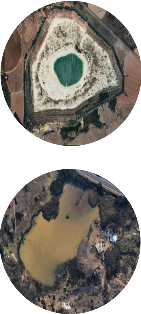
Figure 4.15 AMD Contamination (Google Earth, 2018) Contaminated pools of acid mine drainage.
