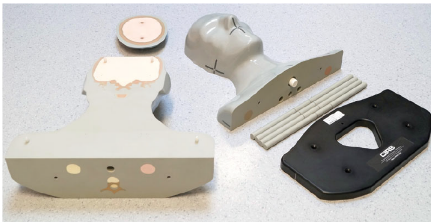
Figure 4: CIRS Shane phantom depicting all elements.
