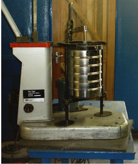
Figures 3.15 & 3.16 – The screen stack loaded into the shaker and the sieves used for screen fractioning the test powder samples.
