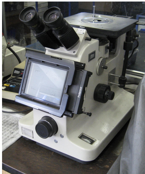
Figure 3.19 – Nikon microscope used to check for porosity
