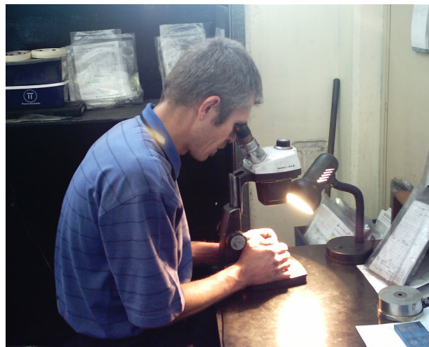
Figure 3.5 – Inspection of green compacts under a stereo-microscope
