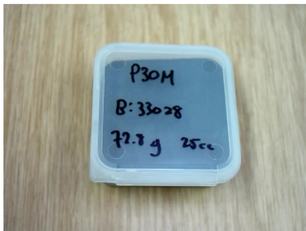
Figure 3.9 – Measured 25 cm 3 and weighed test powder sample in an air-tight container.
