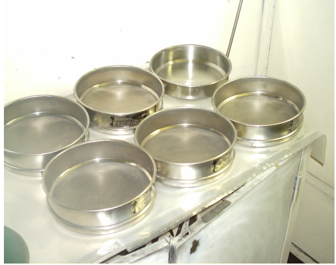
Figures 3.15 & 3.16 – The screen stack loaded into the shaker and the sieves used for screen fractioning the test powder samples.
