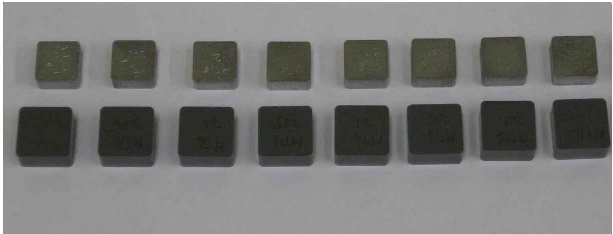
Figure 3.4 – Compacts (bottom) and corresponding sintered pieces (top) of a grade arranged in order from hardest to softest (from left to right) ready for inspection
