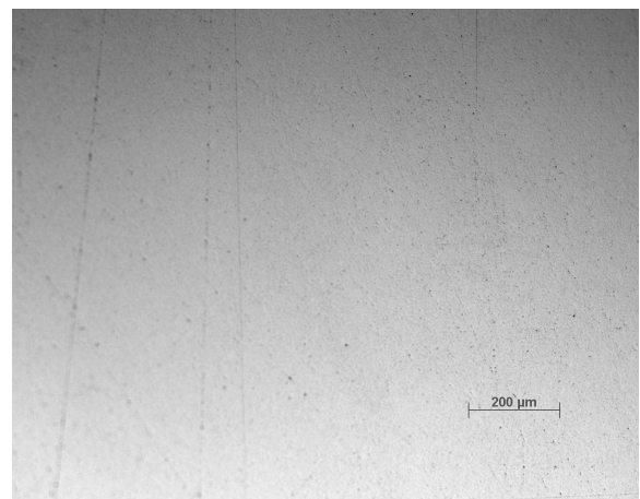
Figure 4.51 – 100x magnification image of polished section of the best shrinkage (least porosity) 20 % and the worst shrinkage (most porosity) 24 % for grade PBT
