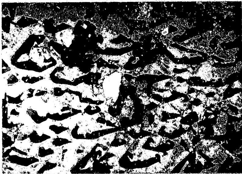
Micrograph of graphic granite (runite). Quartz is in extinction. Light coloured mineral mainly microcline-microperthite. X 22. Crossed nicols. Slide X 4264.
