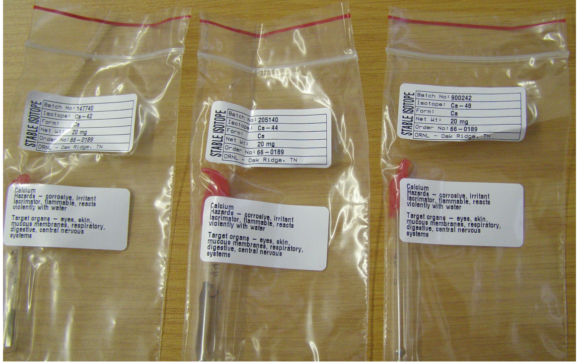
Figure 3.11: The metal pieces of ^{42}\text{Ca} , ^{44}\text{Ca} and ^{48}\text{Ca} (from left to right) prior the rolling.
