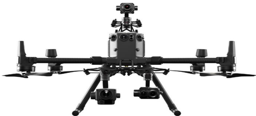
Figure 3-3: UAV equipped with sensors and high-resolution cameras for aerial survey
