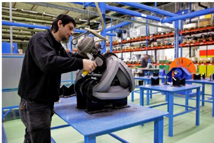
Figure 2: Core assembly of the hexaformer
