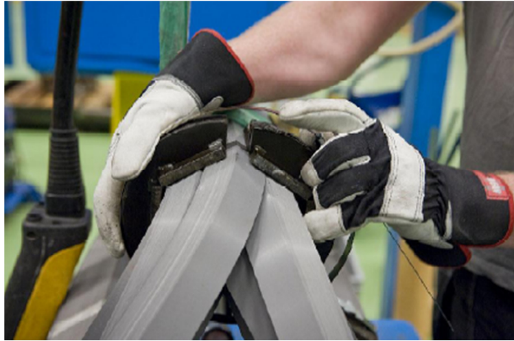
Figure 3: Use of clamps for core assembly
