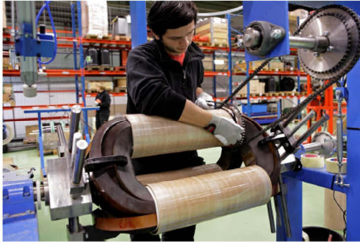
Figure 9: Outer Layer insulation
