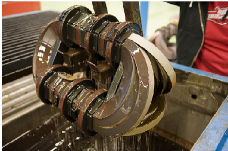
Figure 4: Hexaformer core glued using varnish
