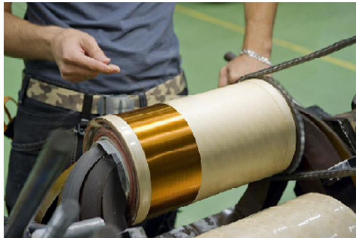
Figure 8: High voltage winding
