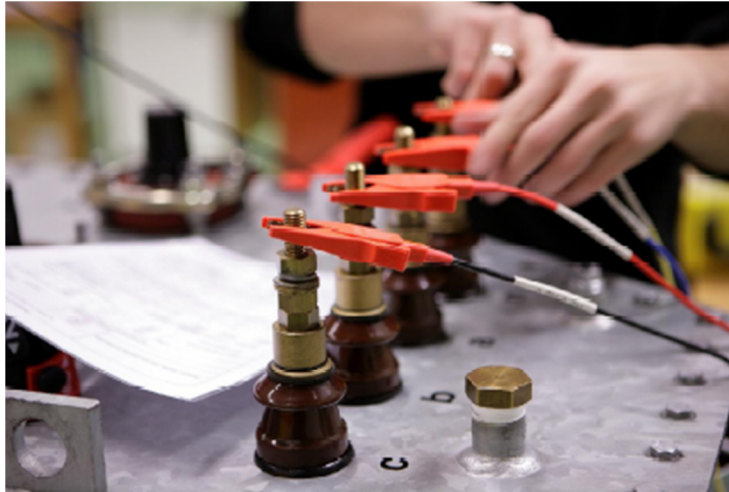
Figure 13: Intermediate in-line electrical test
