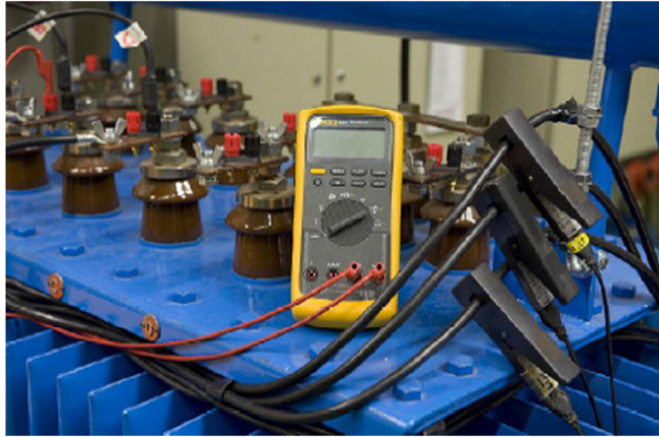
Figure 5: In Line Test of Core Losses
