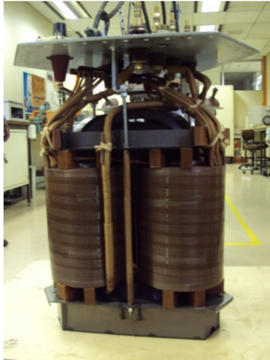
Figure 30: Hexa-transformer unit removed from tank
