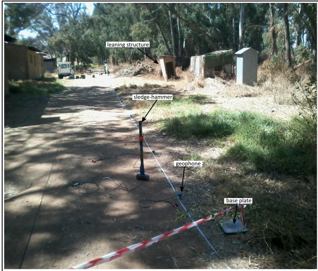
Figure 3.5: A seismic line acquired adjacent to the abandoned leaning structure in the undermined area.
