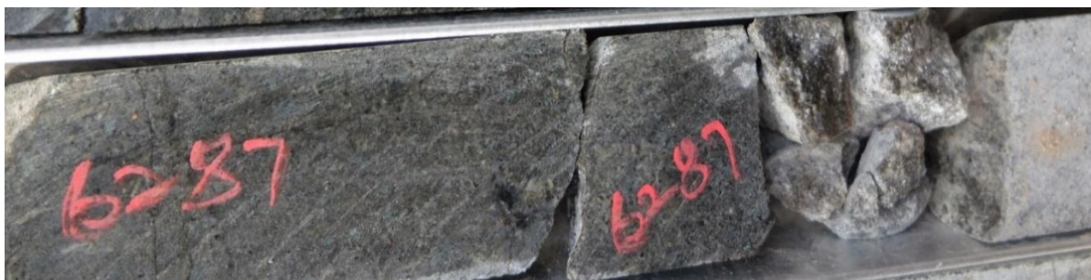
Figure 11-30: A photograph of sample Z20-121.9 (feldspathic pyroxenite).
