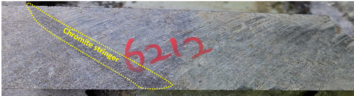
Figure 4-6: A photograph of borehole core sample showing medium to coarse-grained harzburgite (sample Z20-54.25) with a chromite stringer.
