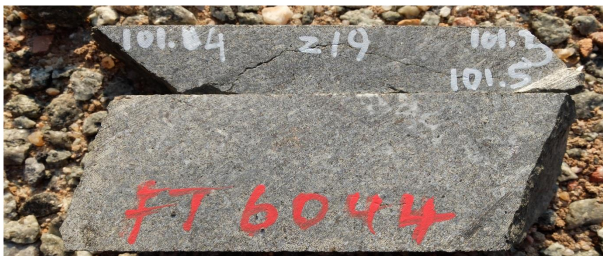
Figure 11-4: A photograph of sample Z19-101. 4 (feldspathic pyroxenite).
