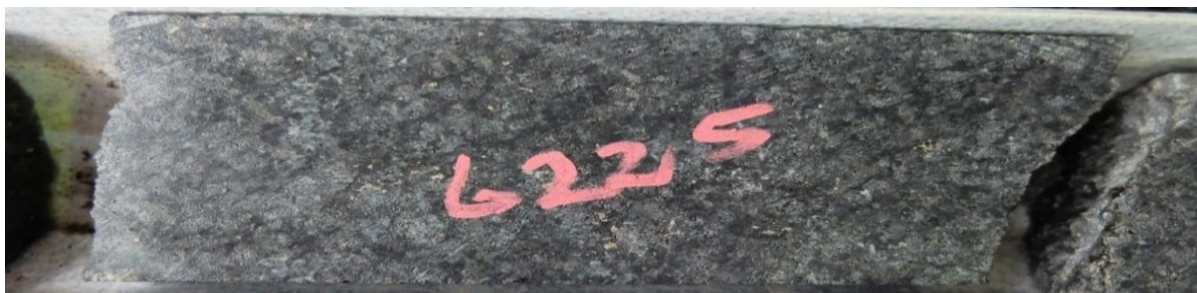
Figure 4-8: A photograph of borehole core sample showing coarse-grained highly serpentinised feldspathic harzburgite (sample Z20-66.5).
