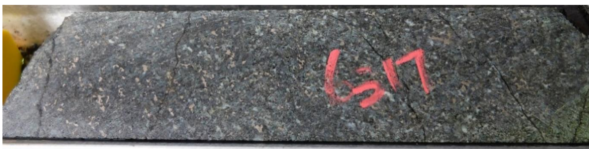
Figure 11-35: A photograph of sample Z20-149.3 (feldspathic pyroxenite).
