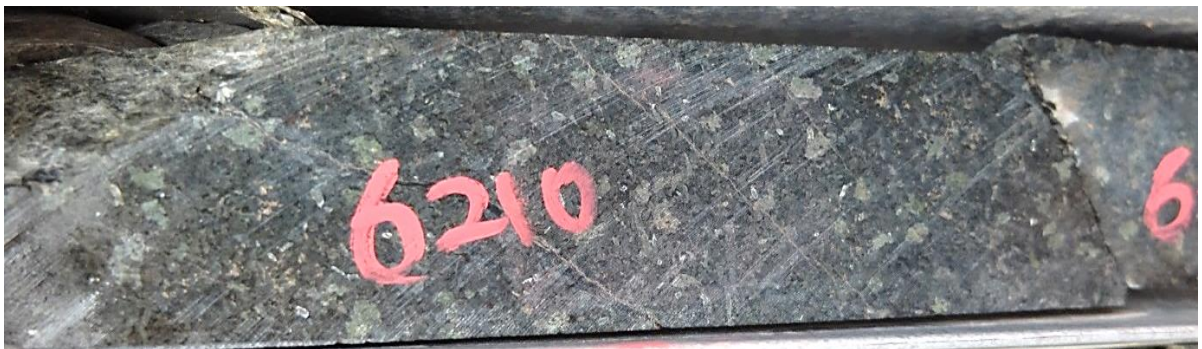
Figure 4-5: A photograph of borehole core sample showing coarse-grained serpentinised harzburgite (sample Z20-53.7).
