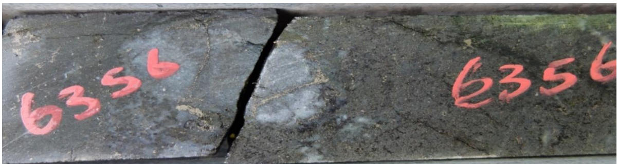
Figure 11-42: A photograph of sample Z20-184.4, hornfels with inclusions of quartz-cordierite hornfels associated with base metal sulphides.
