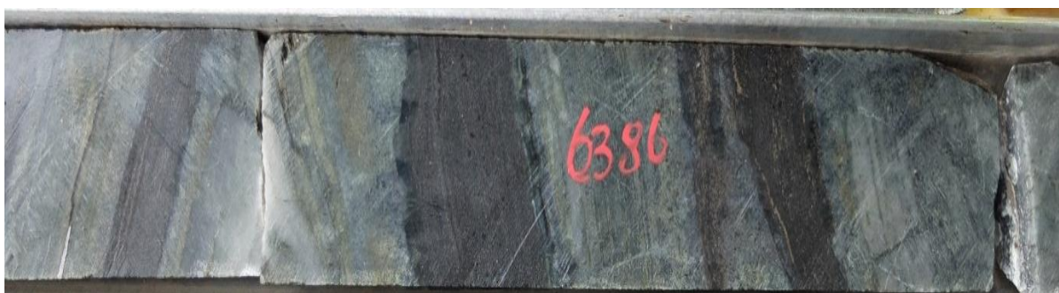
Figure 11-45: A photograph of sample Z20-212.5, dolomite with magnetite bands.
