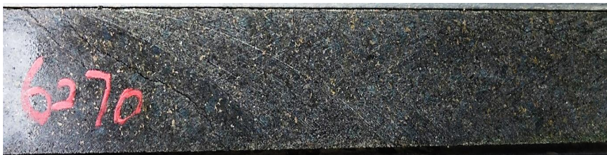
Figure 6-4: A photograph of borehole core samples showing finely disseminated base metal sulphides in feldspathic pyroxenite lithologies at a depth of 107.7 m in borehole Z20.
