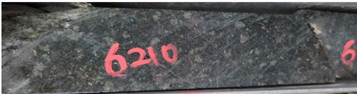
Figure 11-18: A photograph of sample Z20-53.7 (harzburgite).
