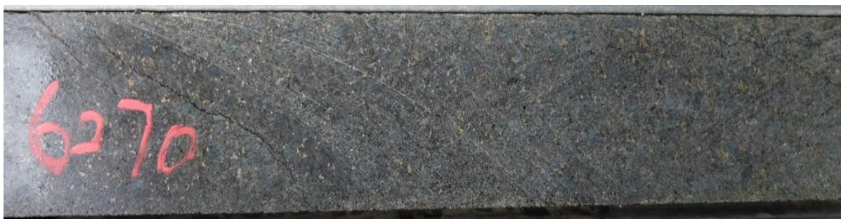
Figure 11-25: A photograph of sample Z20-107.7 (feldspathic pyroxenite).
