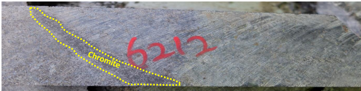
Figure 11-19: A photograph of sample Z20-54.25 (harzburgite with a thin chromite stringer).
