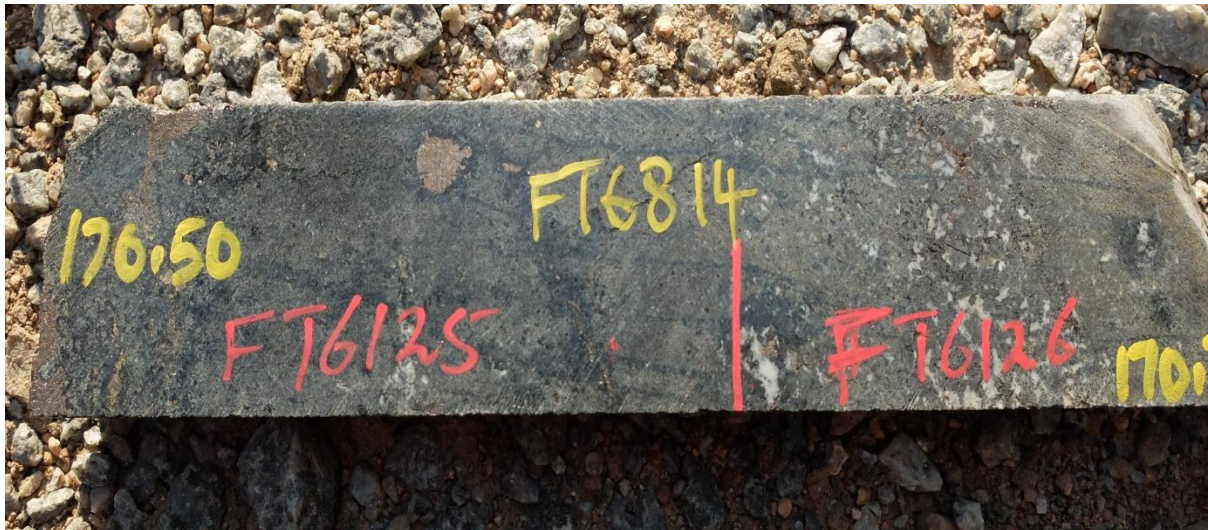
Figure 11-11: A photograph of sample Z19-170.5 (pyroxenite).
