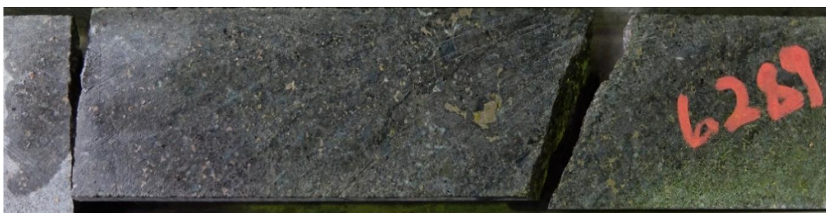
Figure 11-31: A photograph of sample Z20-124.8 (feldspathic pyroxenite).
