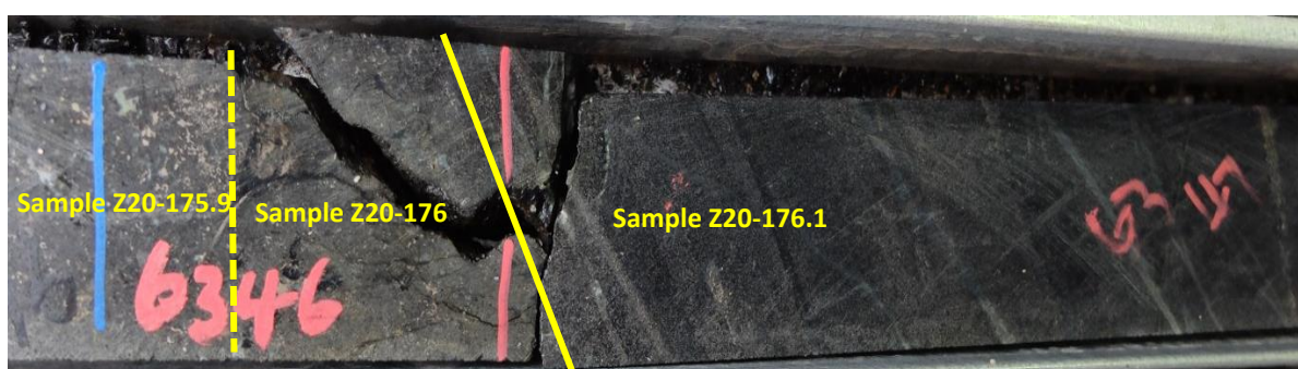
Figure 11-40: A photograph showing a sharp contact between the Rustenburg Layered Suite (RLS) (feldspathic pyroxenite) and the metasedimentary footwall lithologies (hornfels) at a depth of ~176.1m in borehole Z20. A transitional contact is observed between sample Z20-175.9 (feldspathic pyroxenite) and sample Z20-176 (feldspathic pyroxenite).
