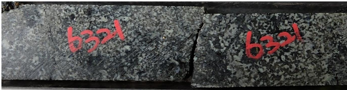
Figure 4-10: A photograph of borehole core sample showing coarse-grained leuconorite (sample Z20-153.5).
