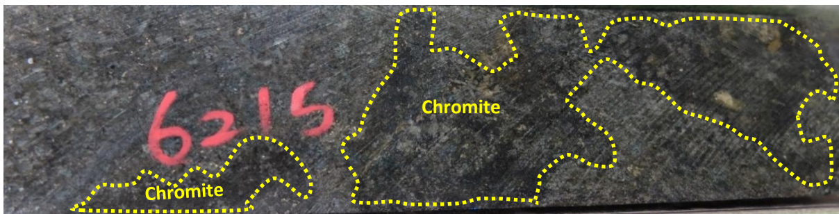
Figure 11-20: A photograph of sample Z20-57.5 (feldspathic harzburgite with chromite disseminations).
