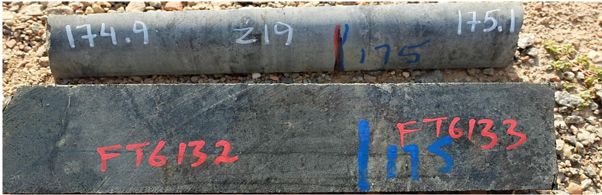
Figure 4-12: A photograph of borehole core sample showing fine-grained parapyroxenite (sample Z19-175.1).
