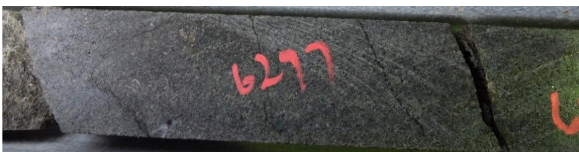
Figure 11-32: A photograph of sample Z20-131.8 (feldspathic pyroxenite).
