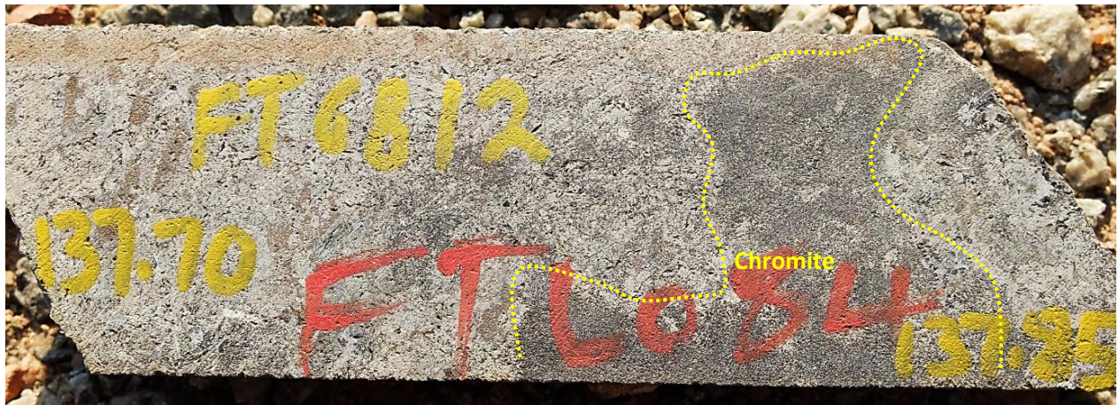
Figure 8-1: A photograph of borehole core sample showing chromite disseminations in feldspathic pyroxenite, sample Z19-137.7.
