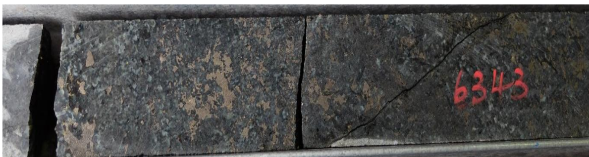
Figure 11-38: A photograph of sample Z20-173.7 (feldspathic pyroxenite).
