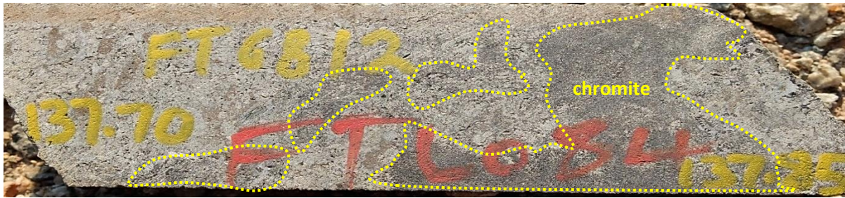
Figure 4-3: A photograph of borehole core sample showing medium to coarse-grained feldspathic pyroxenite (Sample Z19-137.7) with fine-grained chromite disseminations.
