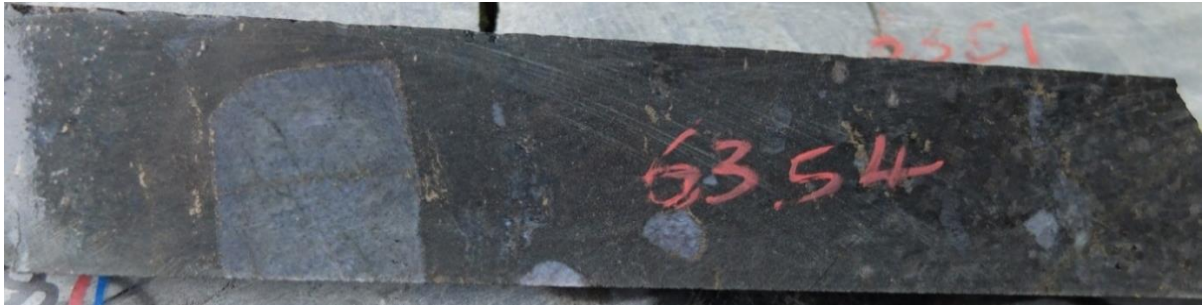
Figure 11-41: A photograph of sample Z20-183.5, hornfels with inclusions of quartz-cordierite hornfels rimmed by base metal sulphides.
