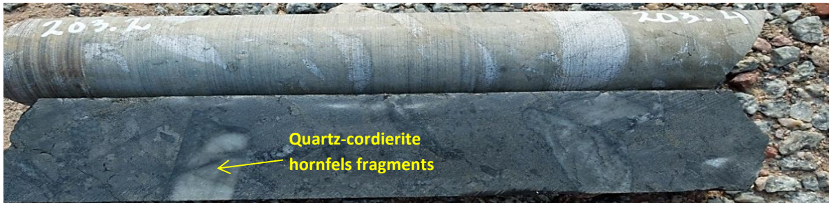
Figure 4-14: A photograph of borehole core sample showing fine-grained hornfels (sample Z19-203.2) with quartz-cordierite hornfels fragments (sedimentary breccia).
