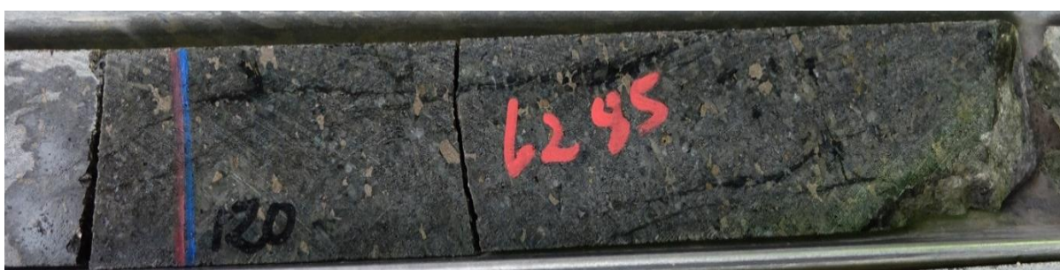
Figure 11-28: A photograph of sample Z20-120.1 (feldspathic pyroxenite).
