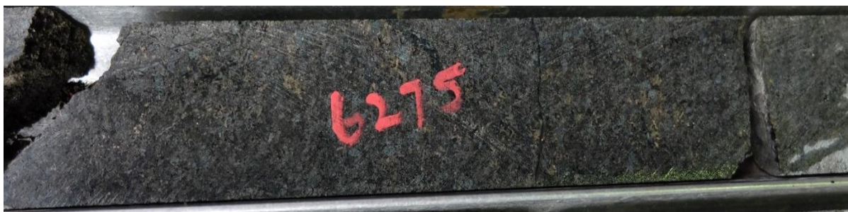
Figure 11-26: A photograph of sample Z20-111 (feldspathic harzburgite).
