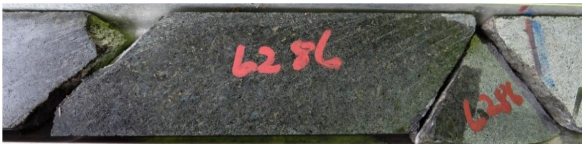
Figure 11-29: A photograph of sample Z20-120.75 (feldspathic pyroxenite).
