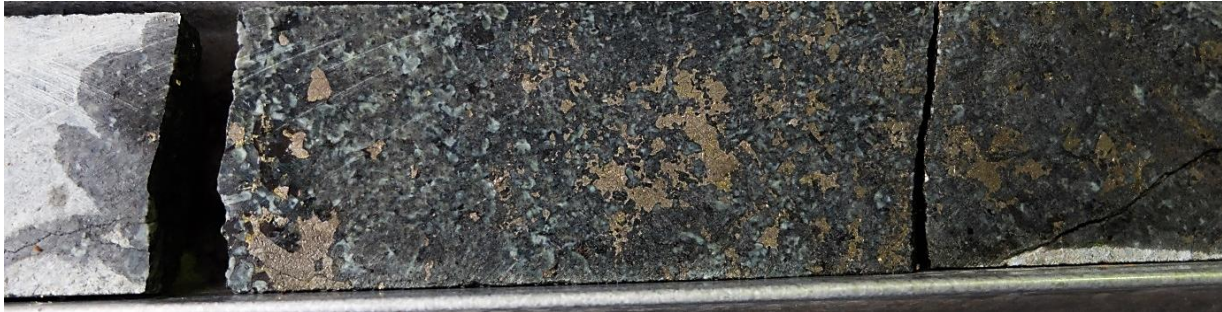
Figure 6-5: A photograph of borehole core samples showing net-textured base metal sulphides, dominated by pyrrhotite, in feldspathic pyroxenite lithologies adjacent to the footwall contact at a depth of ~173.7 m in borehole Z20.
