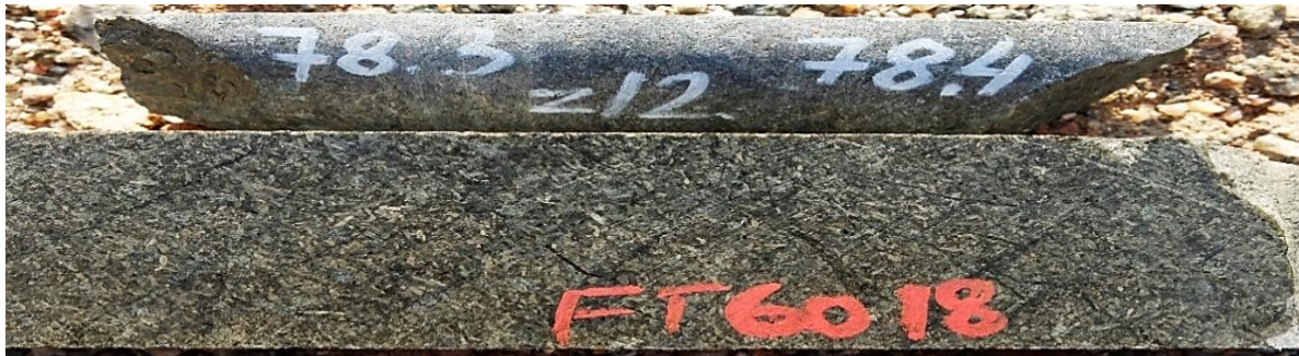
Figure 4-9: A photograph of borehole core sample showing medium-grained melanorites (sample Z19-78.3) with finely disseminated base metal sulphides.
