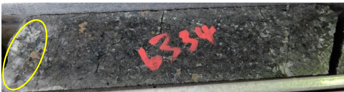
Figure 11-37: A photograph of sample Z20-164.5 (norite with a silica vein).
