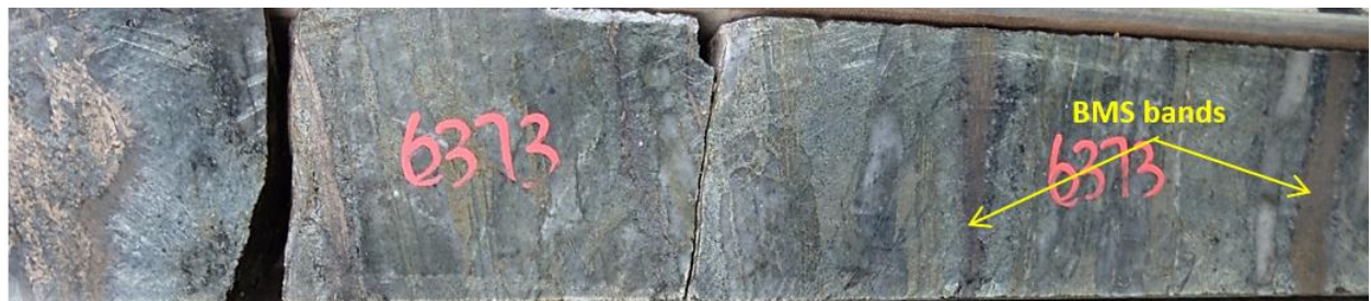
Figure 6-8: A photograph of borehole core sample showing base metal sulphides orientated along bedding structures in calcsilicate lithologies in borehole Z20, where they are associated with magnetite bands.
