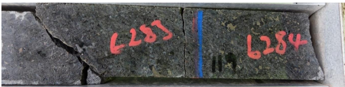
Figure 11-27: A photograph of sample Z20-119 (feldspathic pyroxenite).
