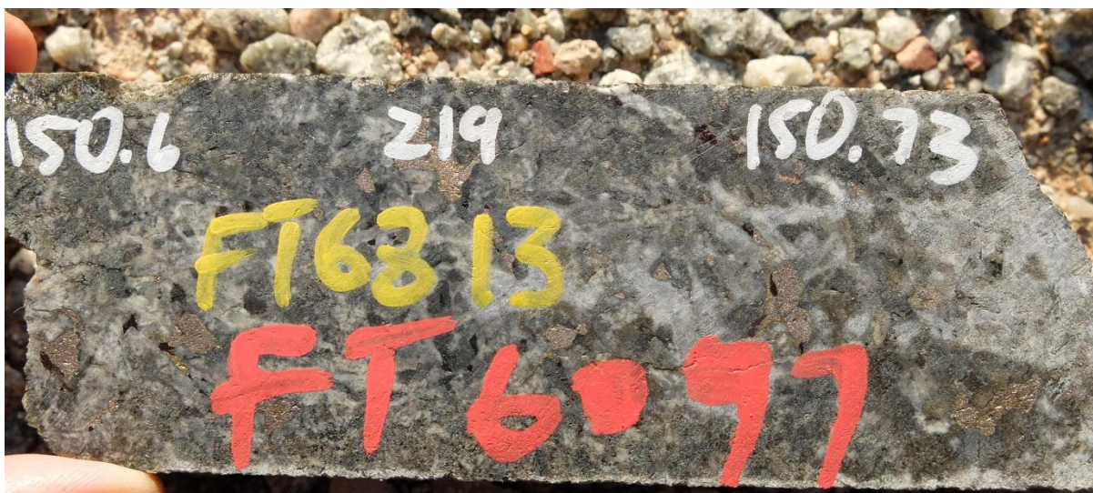
Figure 11-8: A photograph of sample Z19-150.6 (feldspathic pyroxenite).
