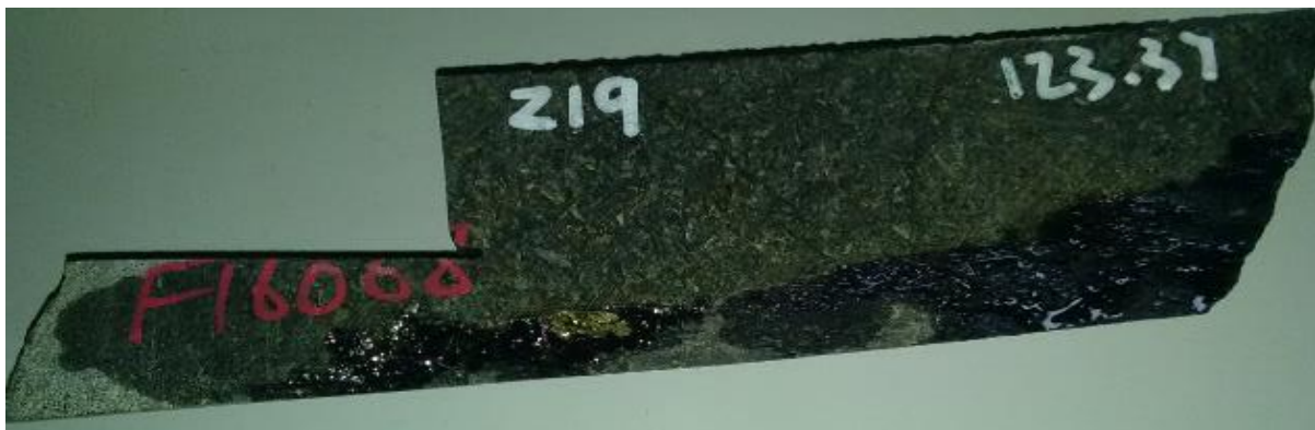
Figure 11-6: A photograph of sample Z19-123.2 (feldspathic pyroxenite).
