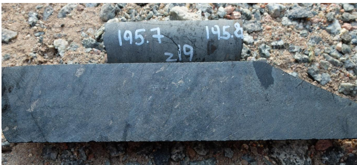
Figure 11-15: A photograph of sample Z19-195.7 (pyroxenite).
