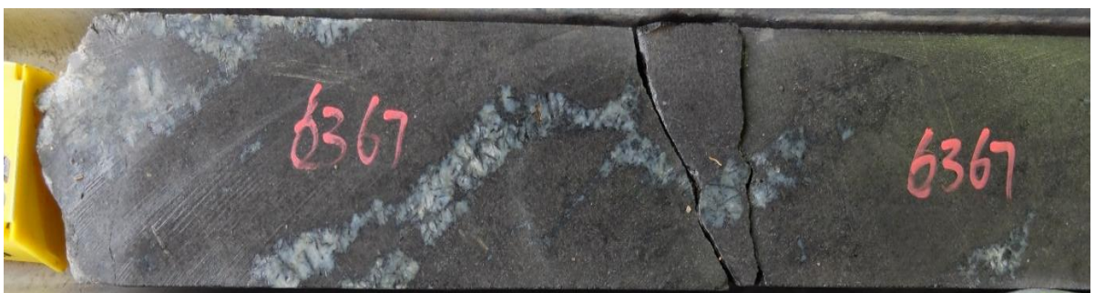
Figure 11-44: A photograph of sample Z20-194.4, hornfels with silica veins.
