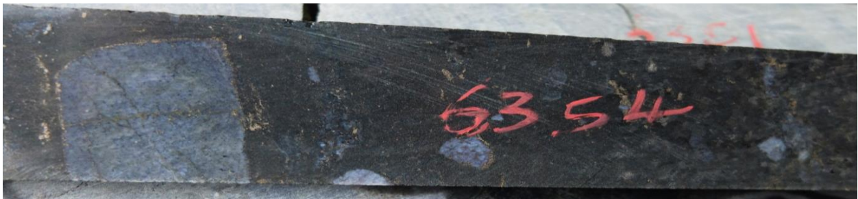
Figure 6-7: A photograph of borehole core sample showing mica-rich hornfels (Sample Z20-183.5), with quartz-cordierite clasts rimmed by pyrrhotite.
