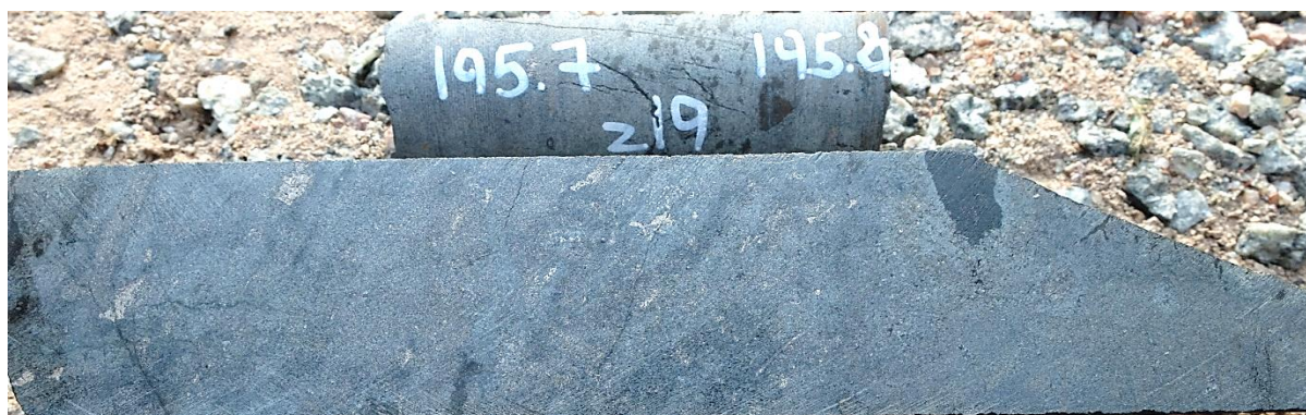
Figure 4-2: A photograph of borehole core sample showing fine-grained orthopyroxenite, sample Z20-195.7.
