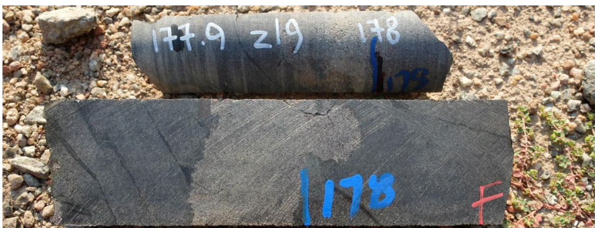
Figure 11-13: A photograph of sample Z19-177.9 (hornfels).
