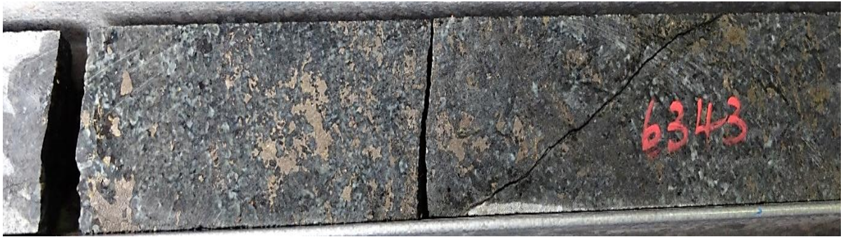
Figure 4-4: A photograph of borehole core sample showing medium to coarse-grained feldspathic pyroxenite (sample Z20-173.7) with net-textured base metal sulphide mineralisation.
