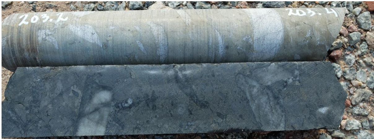
Figure 11-17: A photograph of sample Z19-203.2 (hornfels with calcsilicate inclusions (metasedimentary breccia)).
