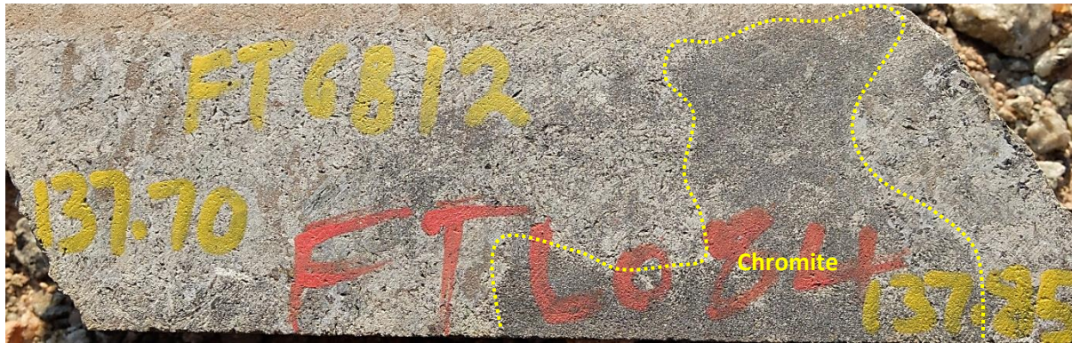
Figure 6-1: A photograph of borehole core samples showing chromite disseminations in feldspathic pyroxenite (sample Z19-137.7).
