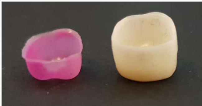
Figure 9: Image showing silicone removed from between the crown and the metal tooth for weighing to calculate the internal fit
