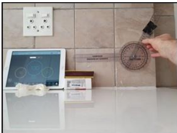
Fig. G 3 Goniometer in 120^{\circ} position with application displaying 130^{\circ} .
