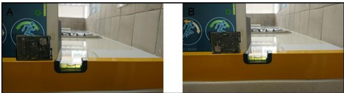
Fig. 4. 2 A) IMU in the upright position with application's spirit level function operating in the background. B) IMU in the inverted position.
