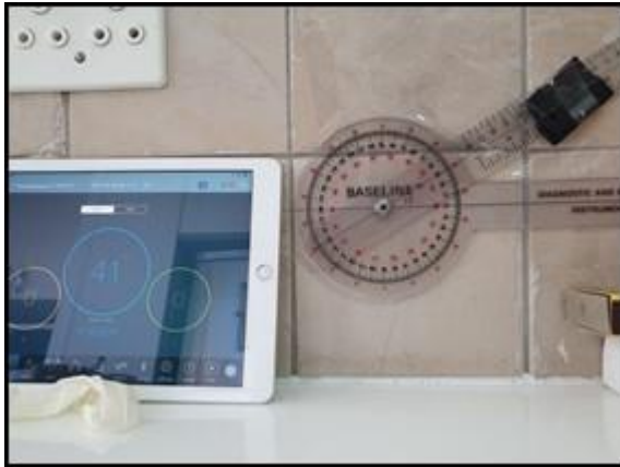
Fig. H 2 The application's angle measurement function displays 41° when the goniometer is positioned at 30°.
