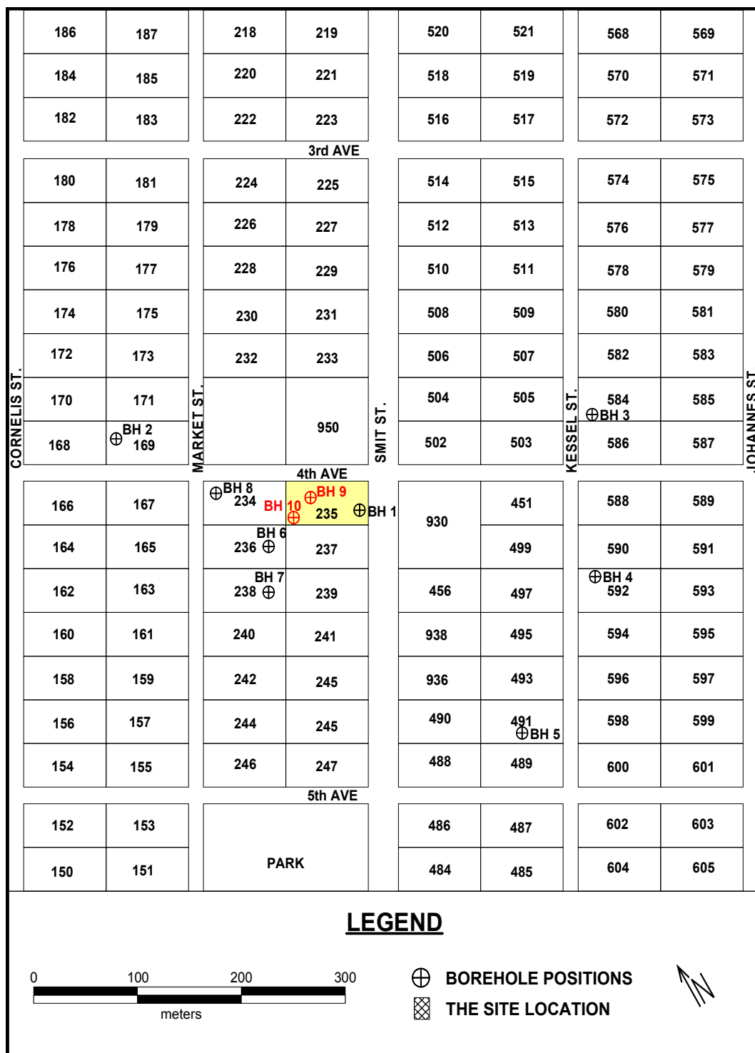
Figure 14: Site Location Map with Borehole (BH) locations indications (Mills and Otten, 2006a)
