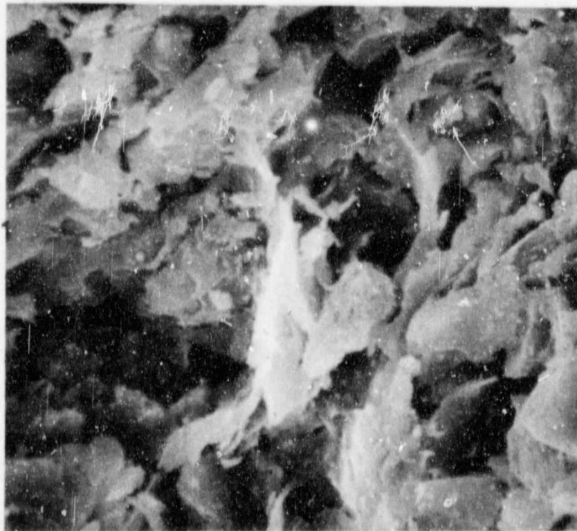
(b) Moisture expansion (1,45 mm/m)
