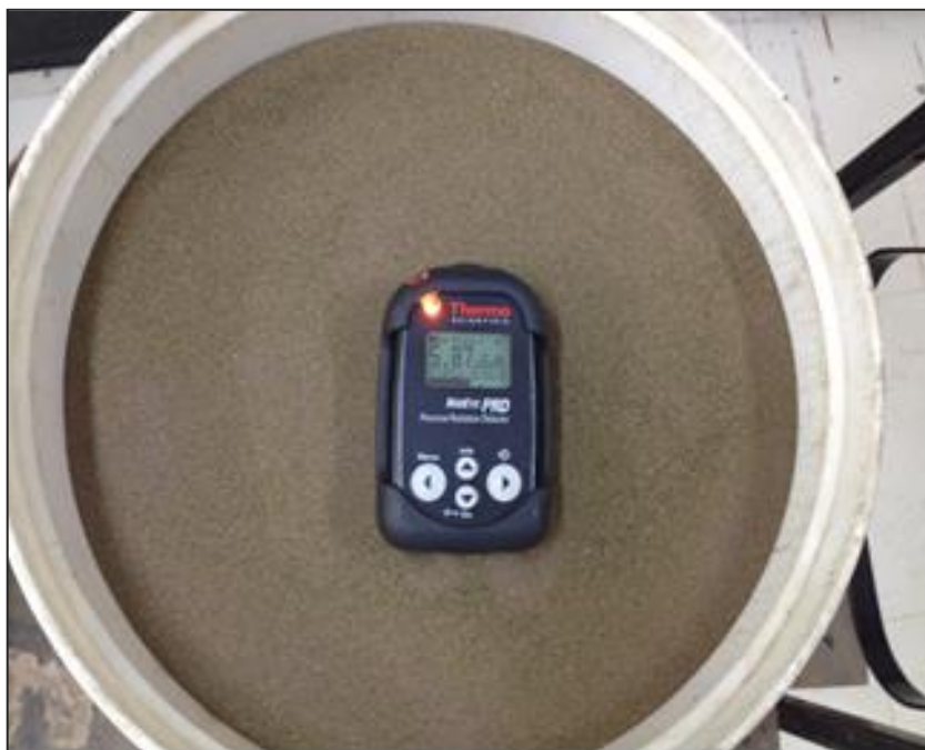
Figure 6: An image showing the 50kg bucket of the research sample, and the recorded radioactive reading of 5.87microsieverts per hour
