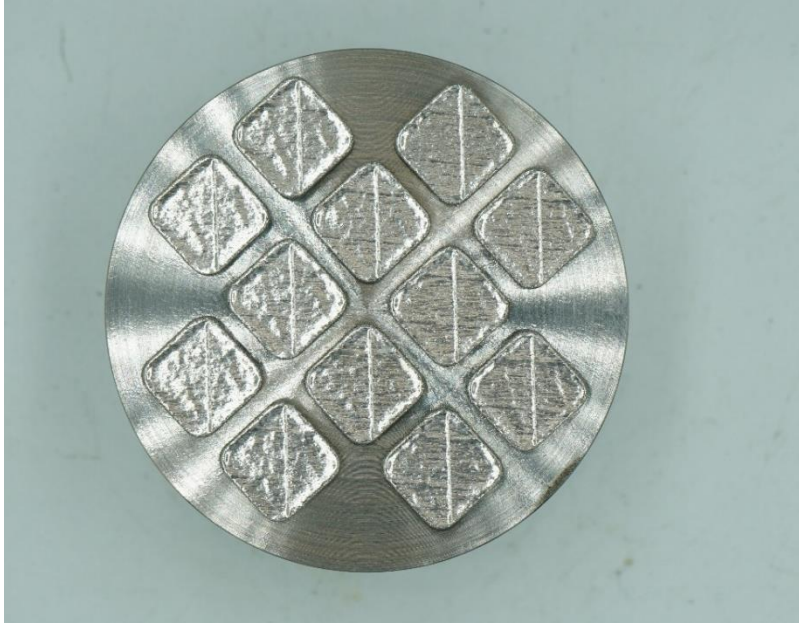
Figure A2.3. Platform after process with selected parameters - top view.
