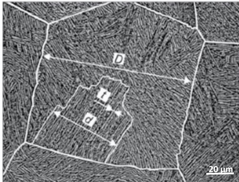
Figure 2.10. SEM-BSE image showing parameters of the lamellar microstructure that was analysed using stereological methods: D = primary \beta grain size, d = size of the colony of parallel \alpha lamellae, t = thickness of \alpha lamellae (Sieniawski et al., 2013).
