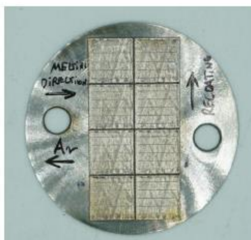
Fig. 2. Photograph of the Ti-6Al-4V substrate disc with 8 LPBF squares supporting 5 horizontal single tracks each, showing directions of argon gas flow, melting and recoating.
