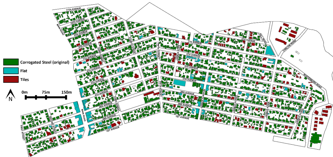
Figure 4.9: Roof types and materials which have an impact on the absorption and reflectivity of incoming solar radiation (Source: Adapted from City of Johannesburg Corporate GIS, Author).
