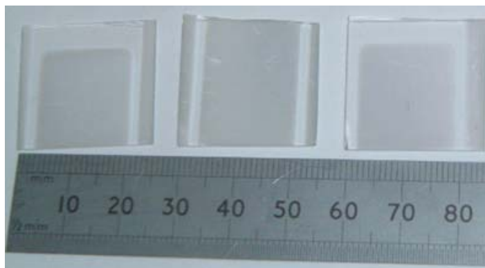
Figure 4.9 \text{TiO}_2 thin films deposited at room temperature, 200 and 400°C on quartz \text{SiO}_2 glass substrate, the films are visually transparent.
