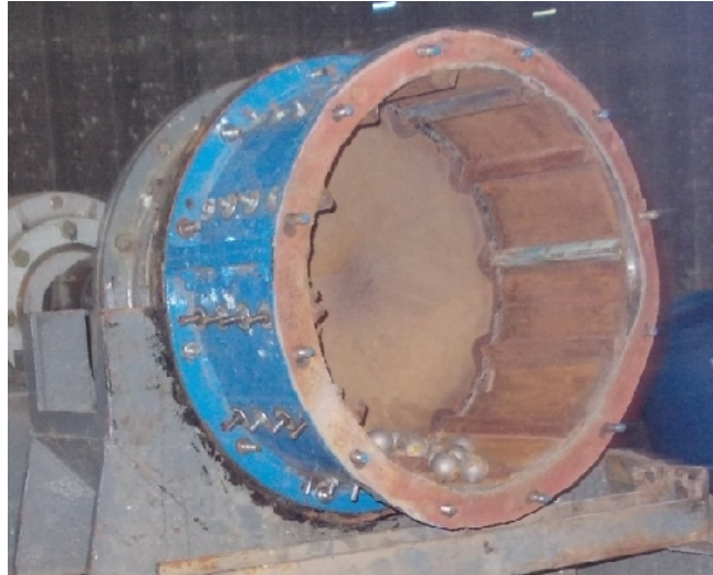
Figure 4.1 Photograph of the laboratory mill showing the lifters attached to one segment of the mill
