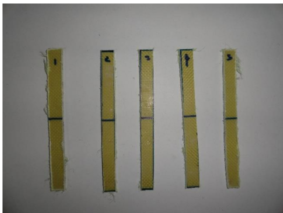
Figure C6: 30% AFC Flexural test specimens (before and after)
