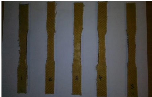
Figure C13: 0.5% CNF doped 0.1% PAN reinforced AFC Tensile test specimens (before and after)
