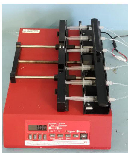
Figure 4-3: NE 1600 Syringe Pump
