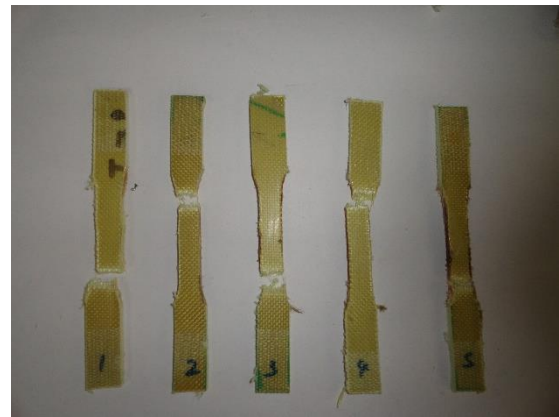
Figure C23: 1% CNF doped 0.5% PAN reinforced AFC Tensile test specimens (before and after)
