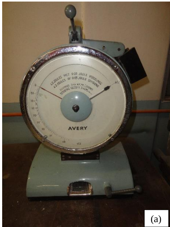
Figure 3-15: (a) - Avery Impact testing machine and (b) - Dimensions of specimen
