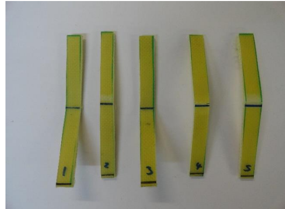
Figure C2: 10% AFC Flexural test specimens (before and after)
