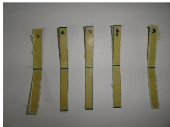
Figure C6: 30% AFC Flexural test specimens (before and after)
