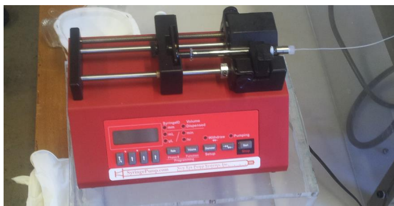
Figure 4-2: NE 1000 syringe pump with metal hub syringe
