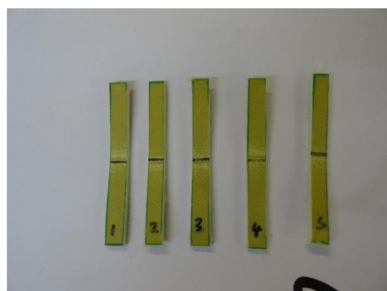
Figure C10: 0.2% PAN reinforced AFC Flexural test specimens (before and after)
