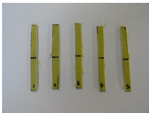
Figure C8: 0.1% PAN reinforced AFC Flexural test specimens (before and after)
