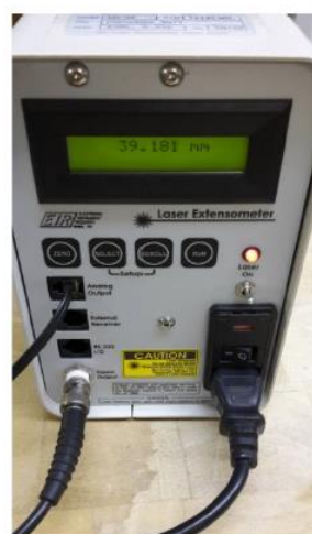
Figure 3-13 Gauge length of sample using the laser extensometer
