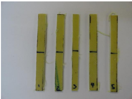
Figure C4: 20% AFC Flexural test specimens (before and after)
