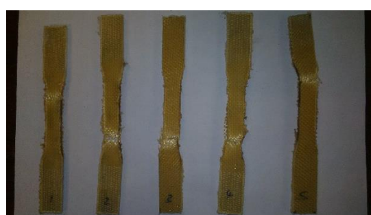
Figure C19: 1% CNF doped 0.1% PAN reinforced AFC Tensile test specimens (before and after)
