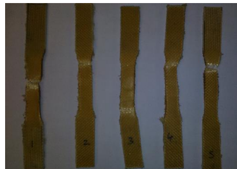
Figure C13: 0.5% CNF doped 0.1% PAN reinforced AFC Tensile test specimens (before and after)
