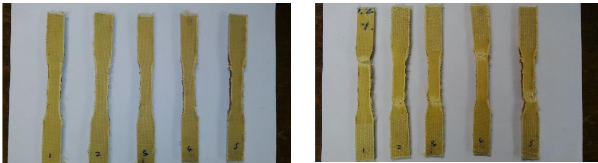
Figure C21: 1% CNF doped 0.2% PAN reinforced AFC Tensile test specimens (before and after)
