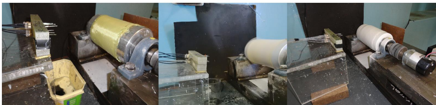
Figure 3-5: Electrospinning PAN onto aramid fibre
