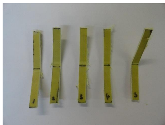
Figure C8: 0.1% PAN reinforced AFC Flexural test specimens (before and after)
