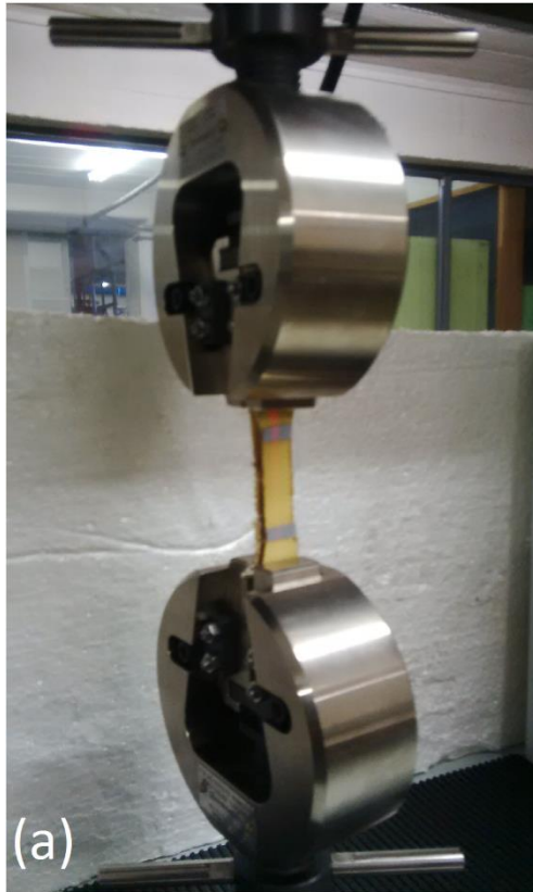
Figure 3-12: (a) Specimen gripped in tensile testing machine and (b) ASTM D3039 dimensions
