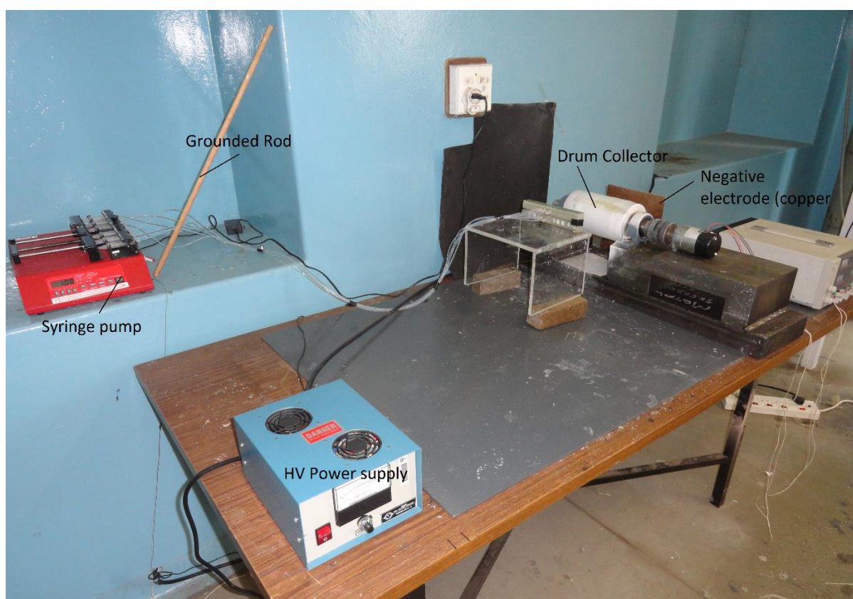
Figure 4-6: Collector design process
