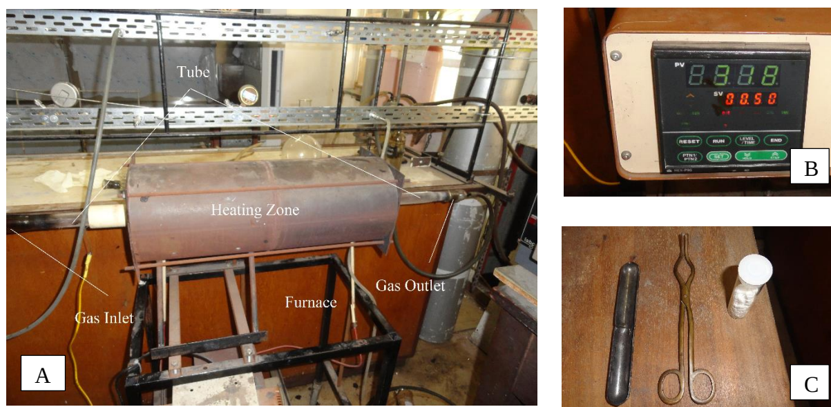
Figure 4-15: (a) - Tube Furnace, (b) - Tube Furnace Temperature Control and (c) - Sample boat, Tongs and PAN nanofibre
