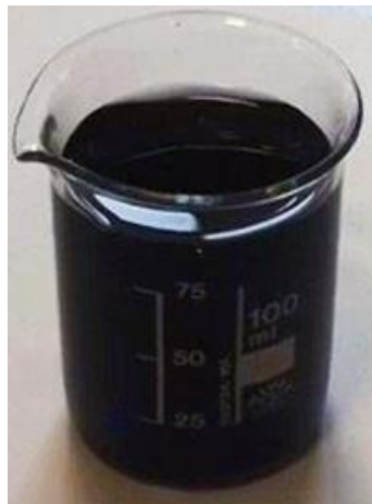
Figure 3-8: Sonicated ECNF/DMF solution.
