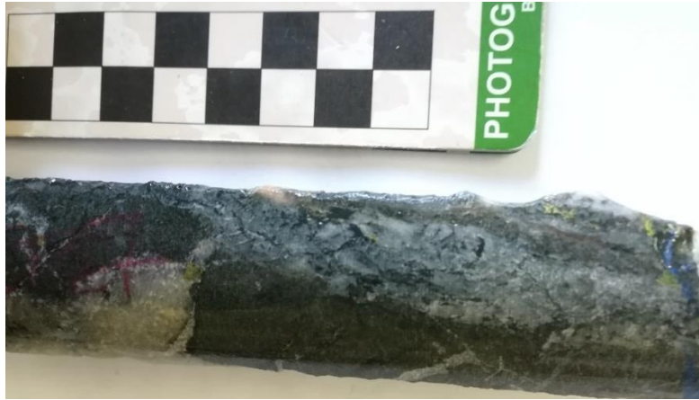
Figure 14: Photograph of the Pienaar Reefs footwalls hand sample that comprises coarse-grained breccia with angular fragments of quartz, carbonates, amphiboles and metabasalts. The hand sample also contains multiple fractures and cross-cutting quartz veins (Borehole P11 at 1302.34 – 132.43 m).
