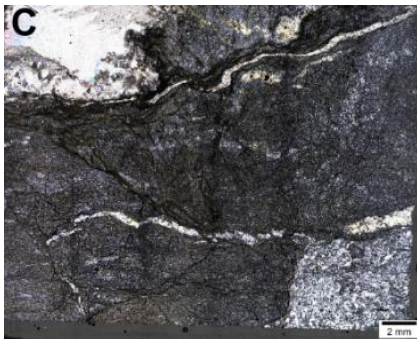
Figure 22: Image showing different structural features associated with quartz veins (1) Boudin structures and (2) Curving quartz veins (Borehole P11 at 130.84 – 131.07 m).
