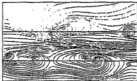
(b) Surface streamline patterns developed from the photograph.
