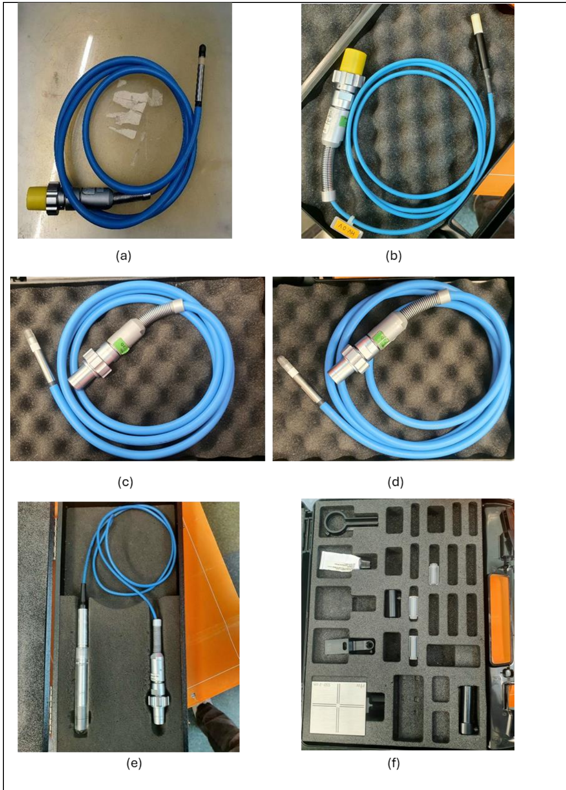
Figure 5: Detectors used: (a) PTW 0.125cm 3 Semiflex (b) PTW 0.004 cm 3 MicroDiamond (c) PTW 0.07 cm 3 Semiflex 3D field (e) PTW 0.07 cm 3 Semiflex 3D reference and (f) TRUFIX BS equipment.
