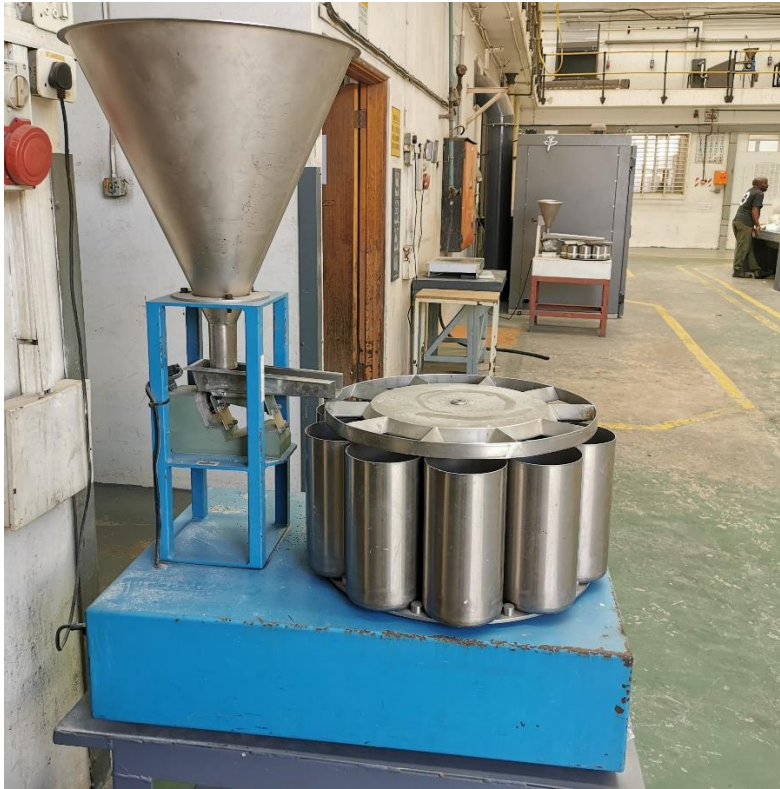
Figure J-3: Rotary Splitter used to divide Sample in Equal Fractions (Mintek)
