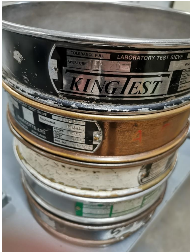
Figure J-5: Sieves used for Particle Size Distribution (PSD) Analysis (Mintek)
