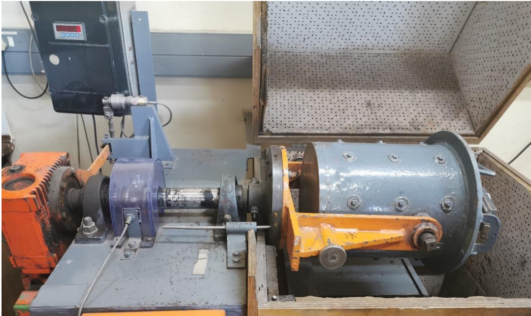
Figure J-13: Ball Mill in Grinding Position (Mintek)
