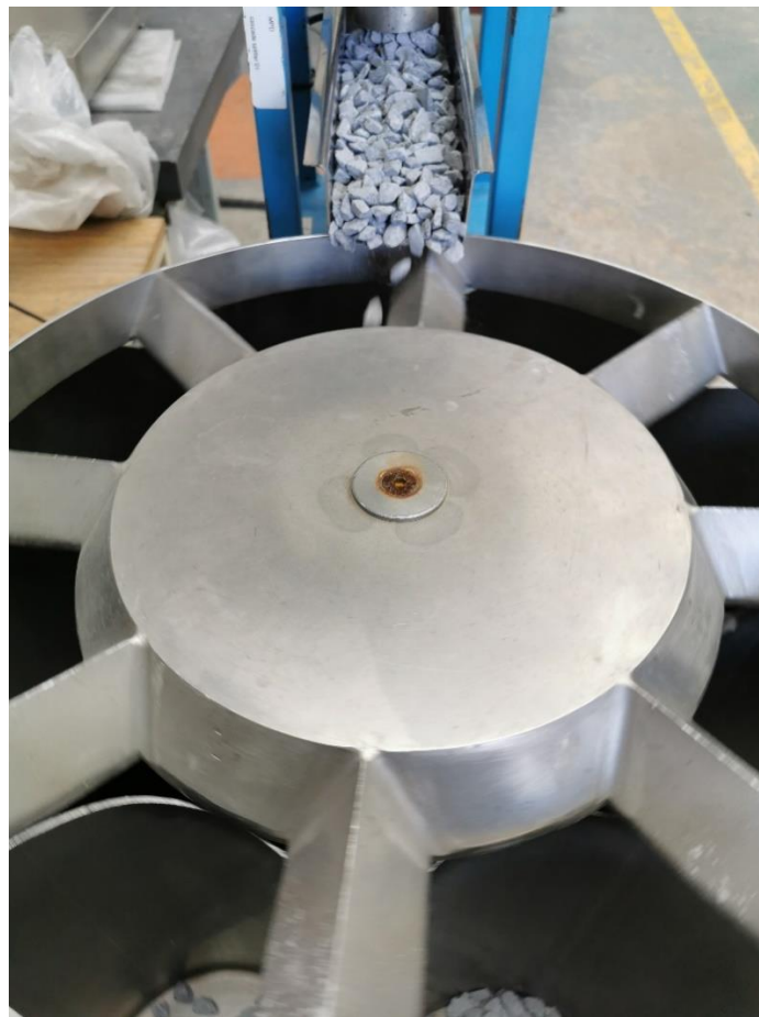
Figure J-4: Rotary Splitter separating Limestone in Equal Fractions (Mintek)
