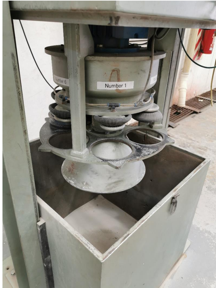
Figure J-7: 6 Pot Swing Mill to Pulverize the Limestone (Mintek)
