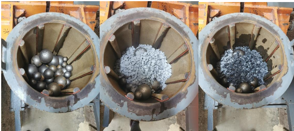
Figure J-12: Ball Mill Filled with (i) Grinding Media, (ii) Grinding Media and Limestone, and (iii) Grinding Media, Limestone and Water (Mintek)
