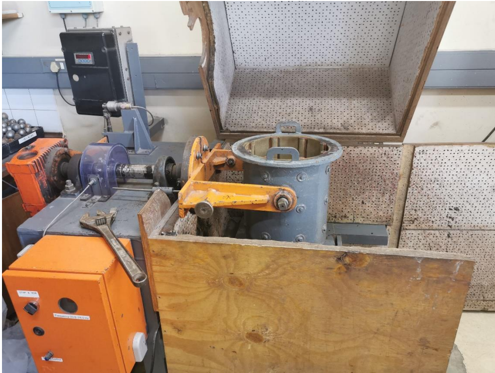
Figure J-11: Laboratory Scale Ball Mill Set-Up Position (Mintek)
