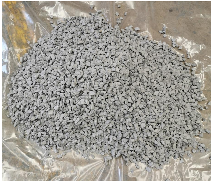
Figure J-2: Limestone Sample -19+8 mm from Danielskuil Idwala Lime
