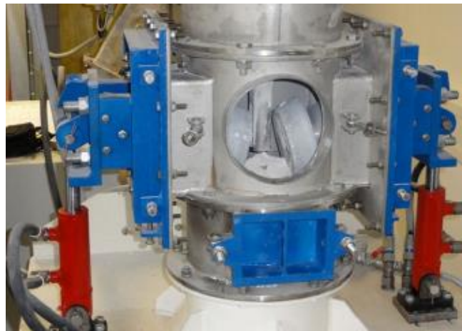
Figure 3-4: Picture of a Laboratory Scale Vertical Roller Mill (Boehm et al., 2015)
