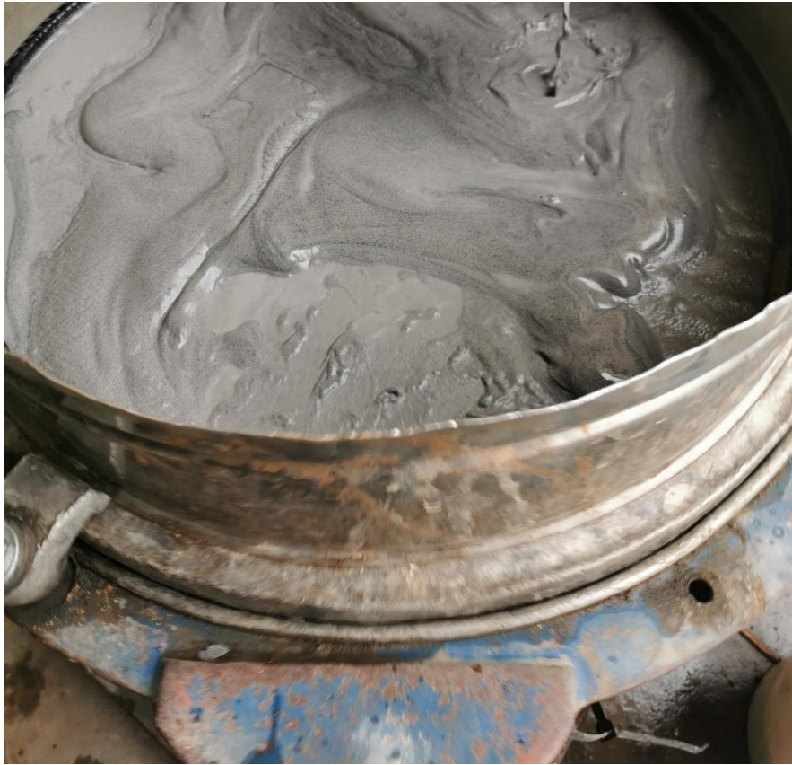
Figure J-15: Roligan with 53 µm Aperture Sieve (Mintek)
