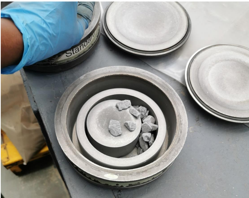
Figure J-8: Grinding Vessels for the 6 Pot Swing Mill (Mintek)
