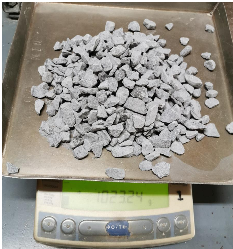
Figure J-6: Laboratory Scale Used for Weighing Limestone during PSD Analysis (Mintek)
