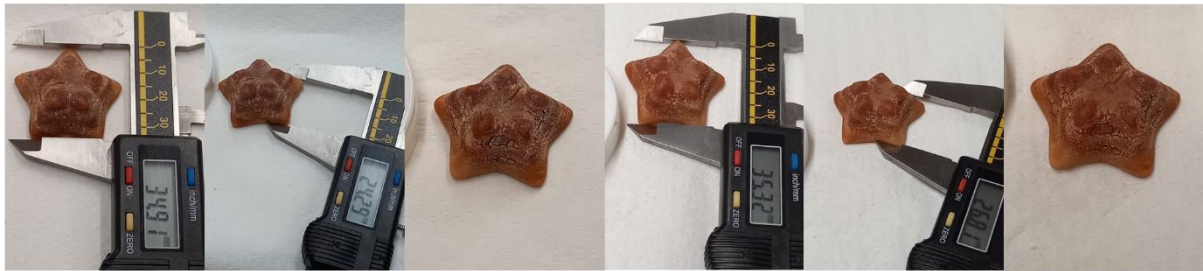
Figure 4.17: ALG-PAAM shape maintenance over time. It can be seen that ALG-PAAM hydrogel implants can maintain its shape after swelling substantially.
