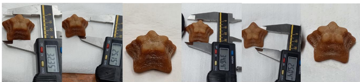
Figure 4.18: BG-ALG-PAAM shape maintenance over time. It can be seen that ALG-PAAM hydrogel implants can maintain its shape after swelling substantially.
