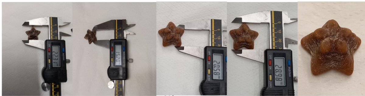
Figure 4.17: ALG-PAAM shape maintenance over time. It can be seen that ALG-PAAM hydrogel implants can maintain its shape after swelling substantially.
