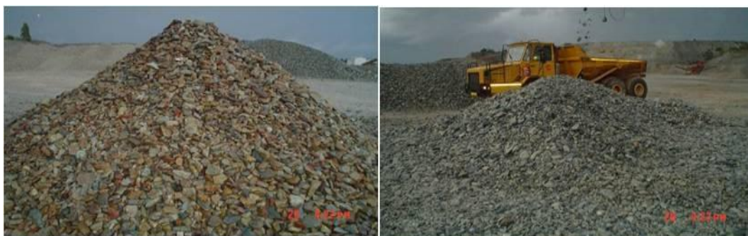
Figure 24. Optical sorter product (left) and sorter discard (right)
