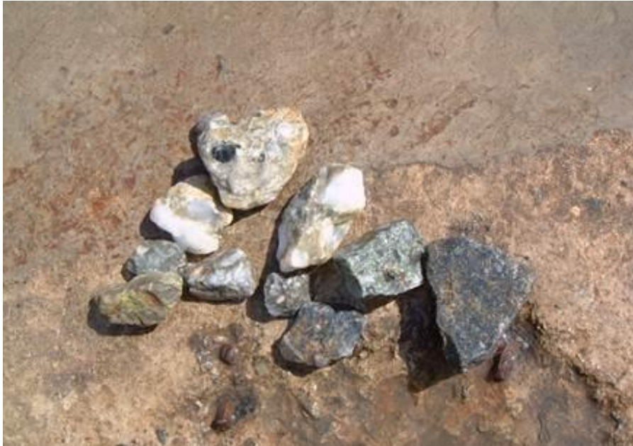
Figure 16. Gold reef not detected by the optical sorter
