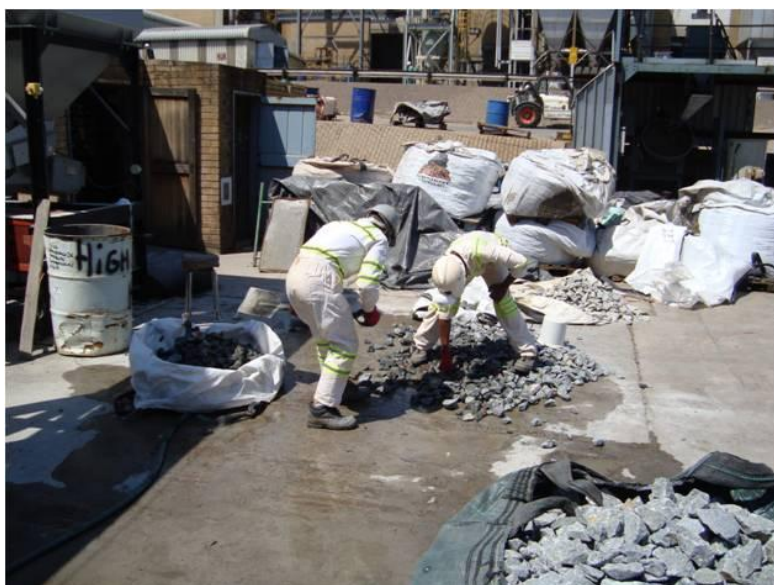
Figure 38. Evaluation of sorted fractions by hand sorting
