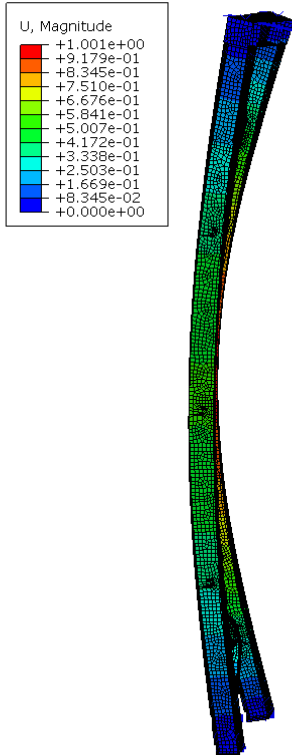
Figure 4:38 Buckled finite element model when the load ratio ( P/N ) > 1
