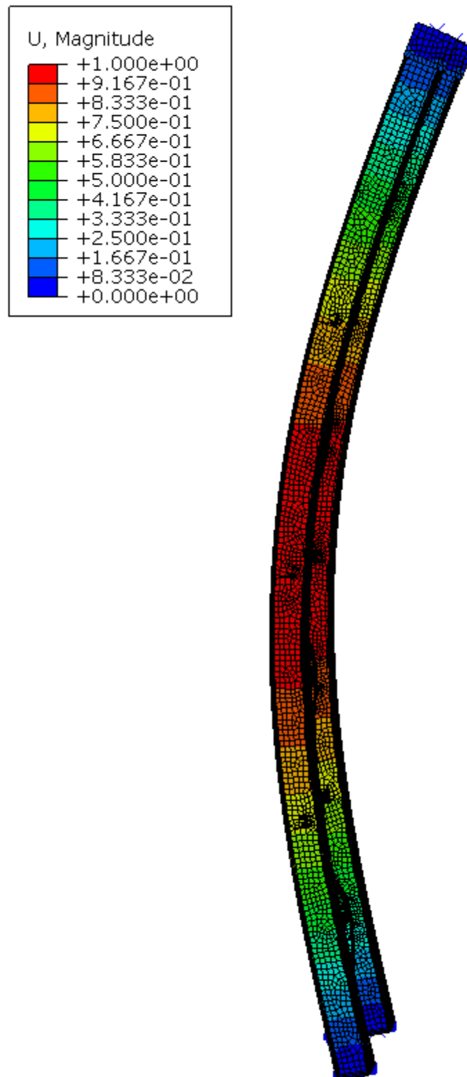
Figure 4:37 Buckled finite element model when the load ratio ( P/N ) is \pm 1
