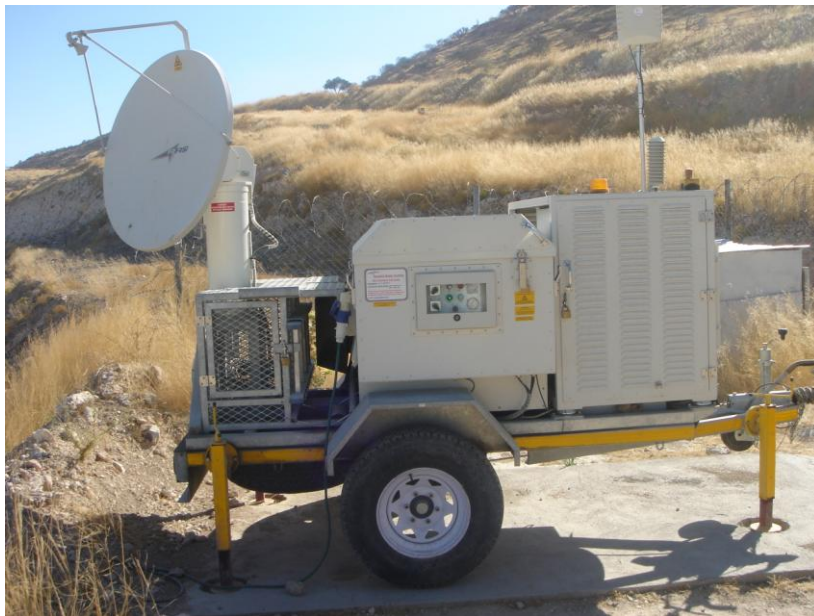
Plate 4 - Slope stability radar – deployed
