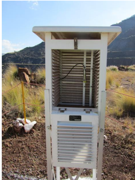
Plate 20 - Stevenson Screen with meteorological sensor for measuring ambient temperature and atmospheric pressure
