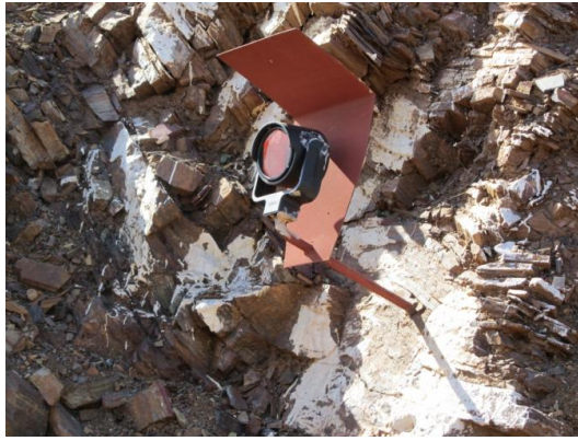
Plate 14 - Monitoring prism attached to bench face or highwall
