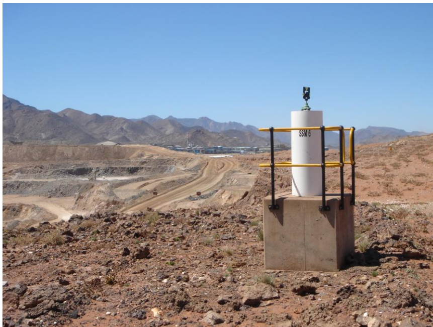
Plate 21 - Pillar type (forced centring) reference beacon for slope stability monitoring
