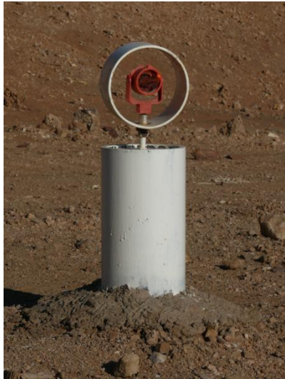
Plate 25 - Protected crest prism for slope stability monitoring
