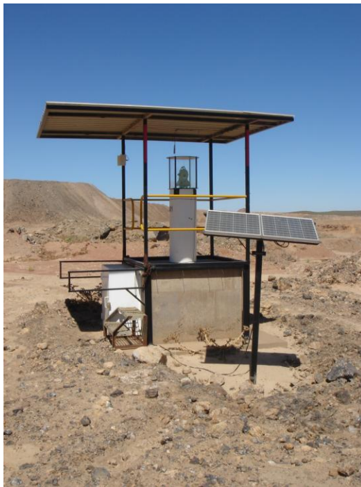
Plate 1 - Transfer beacon located on elevated platform to allow for line-of-sight into the open pit
