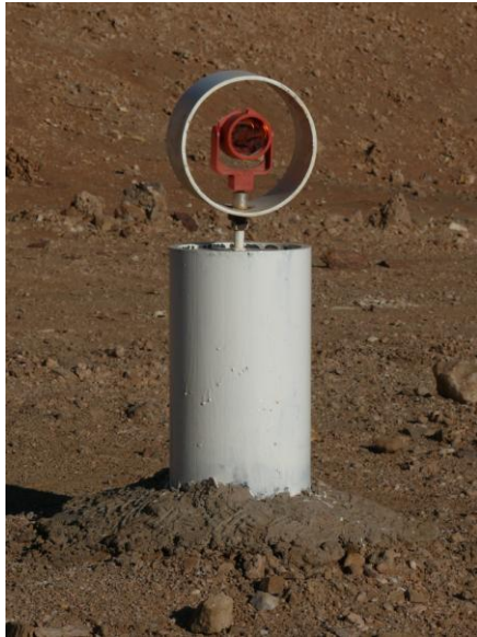
Plate 16 - Bench crest type monitoring point prism with steel rod support encased in concrete filled pipe to mitigate the affect of the wind
