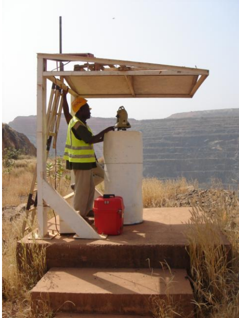
Plate 22 - Protective shade canopy for slope stability monitoring instrument and beacon
