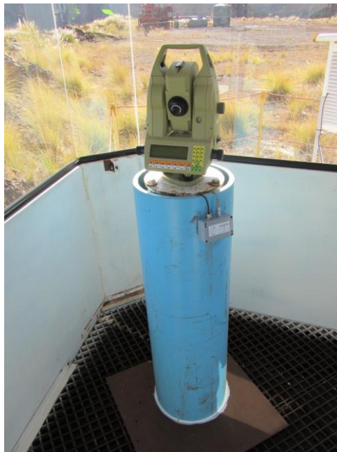
Plate 8 - Transfer beacon with plastic pipe casing to mitigate the effect of the heat of the Sun on the pillar
