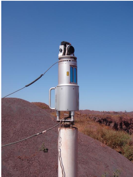
Plate 3 - Laser scanner mounted on survey pillar beacon
