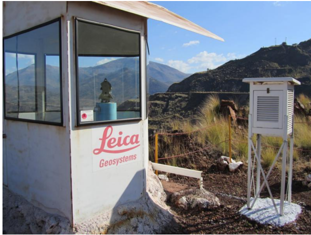
Plate 24 - Protective housing for slope stability monitoring instrument with Stevenson Screen
