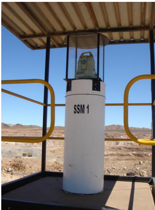
Plate 23 - Protective housing and shelter for slope stability monitoring instrument
