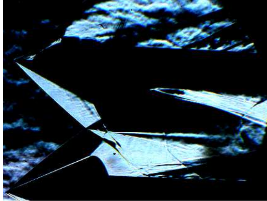
Figure 4.6: Example of a schlieren image taken with optical yaw with a free-stream Mach number of M_1 = 3.0 .
