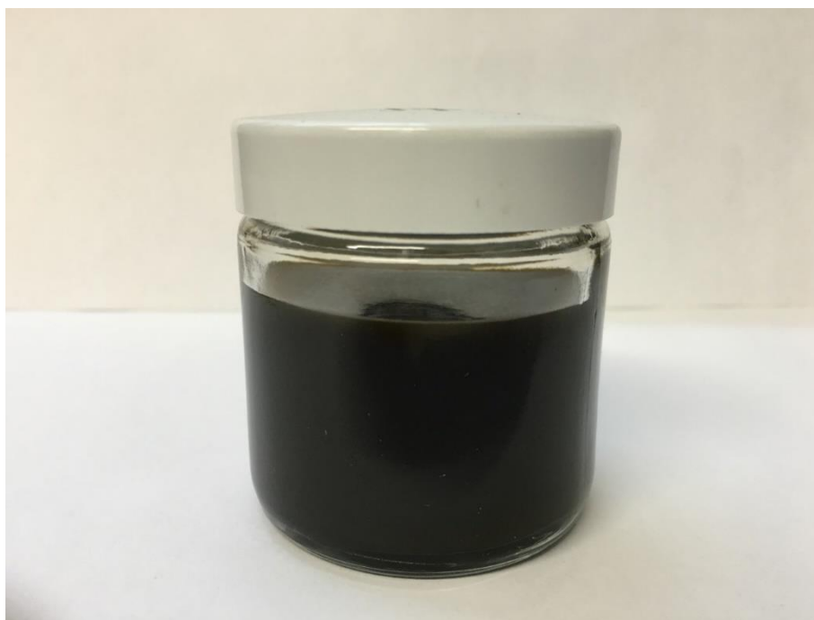
Figure 7.1 Product formed during solvothermal reaction of sucrose and HILG13 < 32µm
