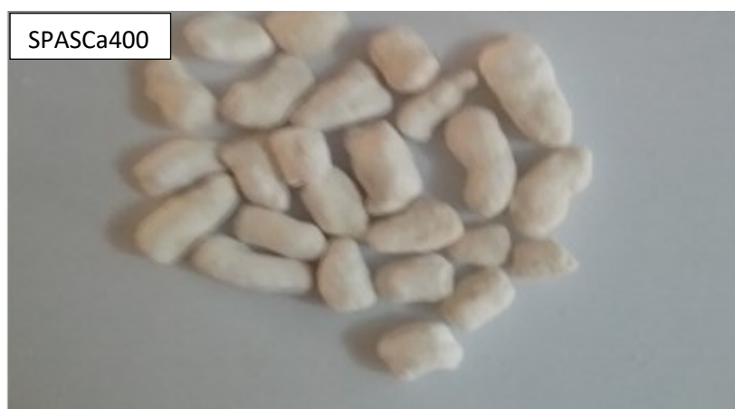
Figure 2.9 The photograph of the synthesized cylindrical-shaped and calcium promoted SPASCa400 catalyst synthesized from synthetic kieselguhr and calcined at 400 °C.
