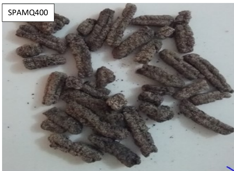
Figure 2.7 The photograph of the synthesized quadrilobed shaped SPAMQ400 catalyst calcined at 400 °C and synthesized using mined kieselguhr showing distinct quadrilobed shaped extrudates with all four vertices.
