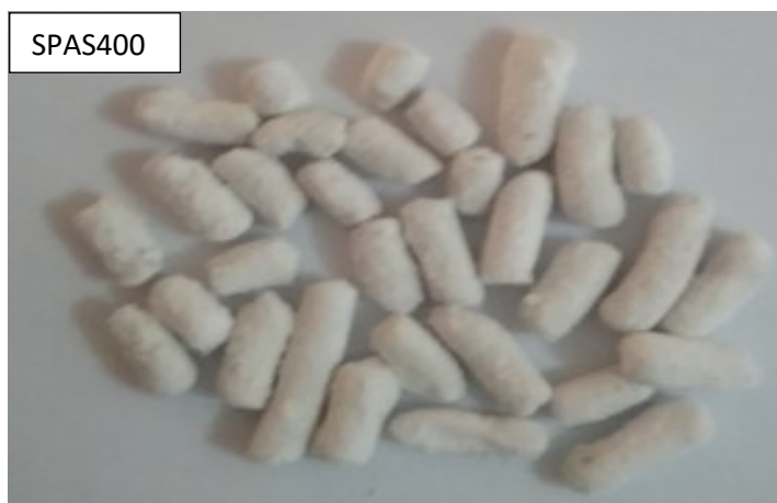
Figure 2.8 The photograph of the synthesized cylindrically shaped SPAS400 catalyst synthesized from synthetic kieselguhr, the catalyst is cylindrically shaped just like the SPAMT catalyst series.
