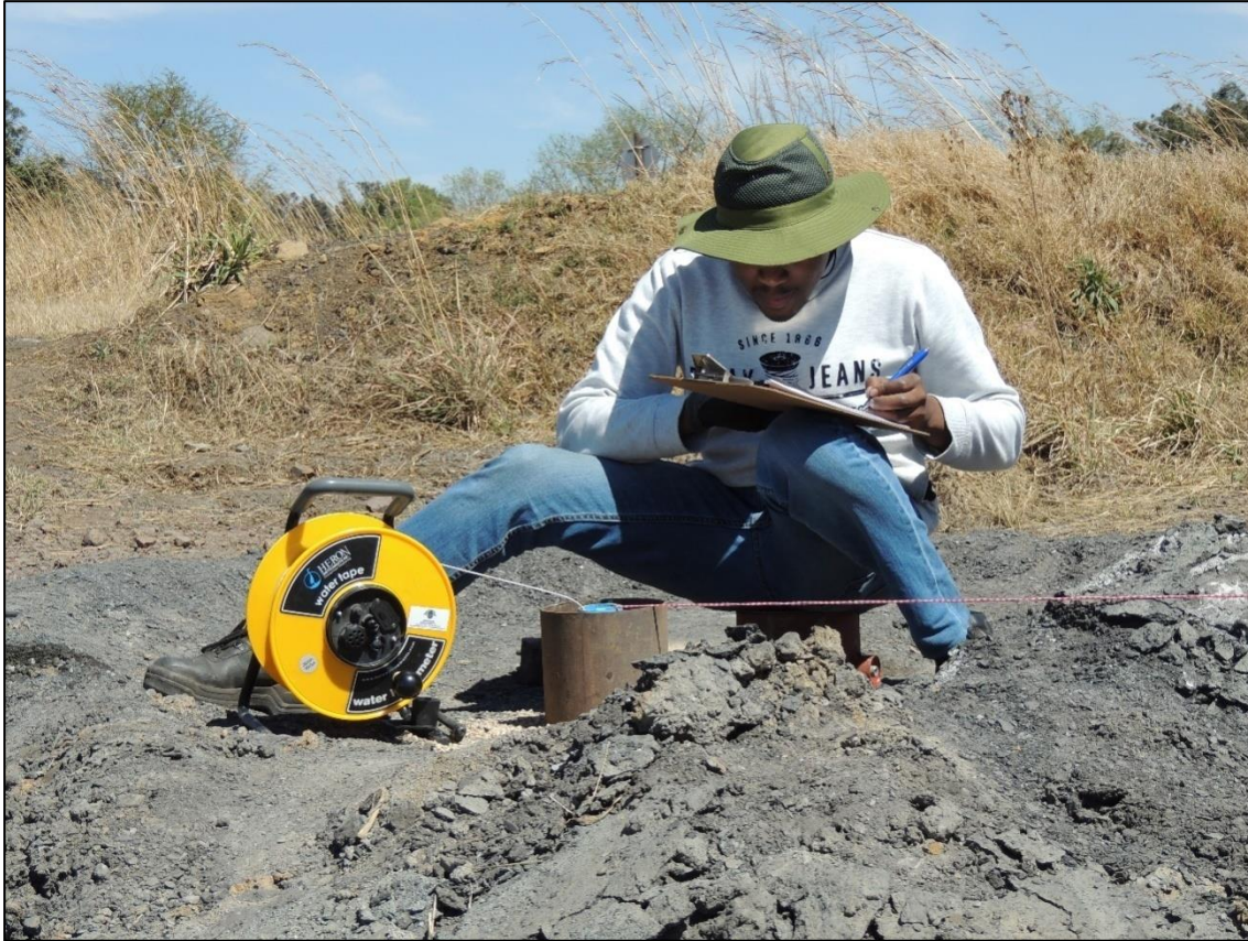
Figure 4-4: Slug testing borehole 1 (BH01) on the study location.
