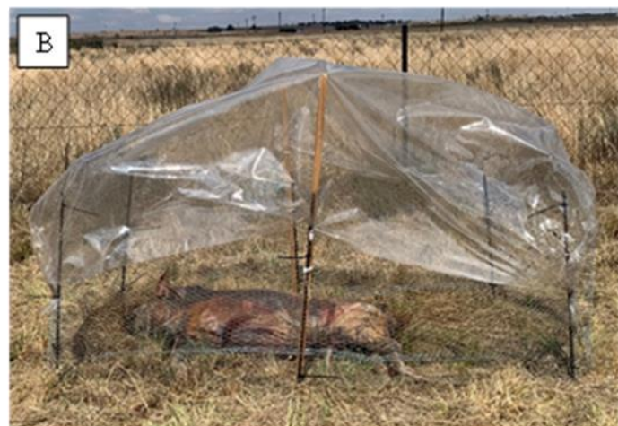
Figure 4.2: Secondary cages, constructed with mesh and iron rods covered with a plastic tarp. A) A side profile displaying cage breadth and height, and B) front profile of cage displaying cage width and height and connection of tarp with space for airflow.
