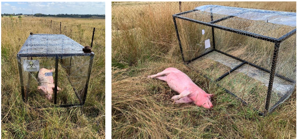
Figure 3.2: Custom metal cages, 0.9m x 0.9m x 2.0m, surrounded with chicken mesh wire to prevent the entry of large scavengers and covered with a transparent plastic tarp, fastened to the cage, to prevent natural rehydration.
